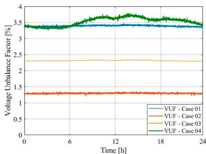
**Figure 7.** Voltage unbalanced factor at the PCC for simulated cases.
