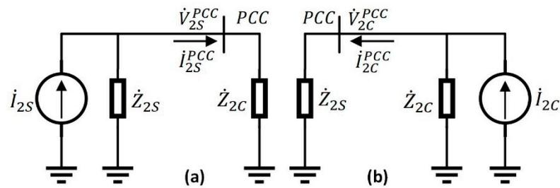
**Figure 2.** Norton equivalent circuit: (a) contribution originating from the supplier; (b) contribution from the consumer.
