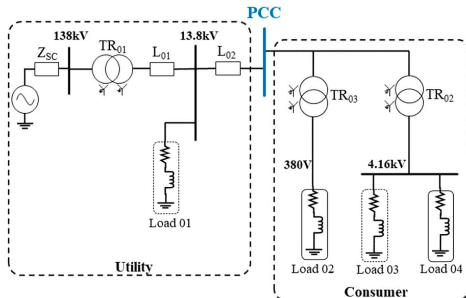
Figure 5. Electrical system used for the studies.
