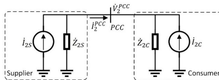
Figure 1. Norton equivalent circuit of negative sequence.
