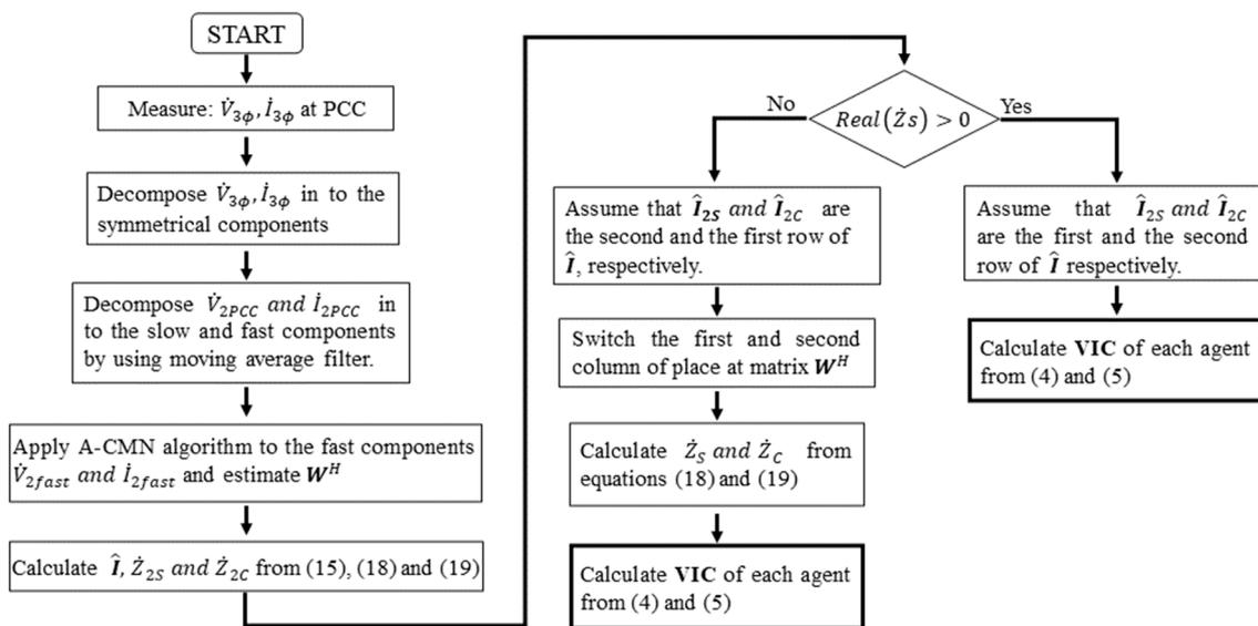
Figure 4. Flowchart of the CICA method for determining voltage imbalance contributions.
