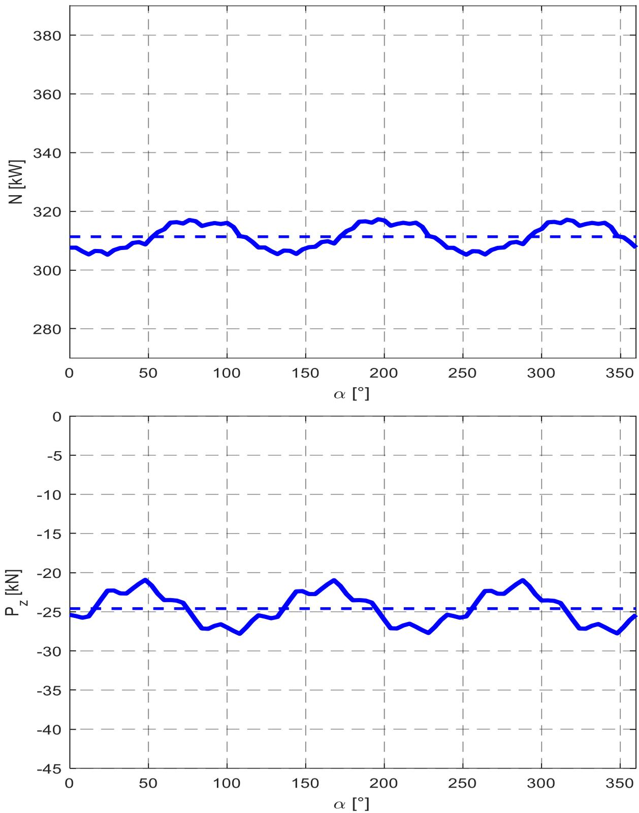
**Figure 13.** Waveform of the values of power  $N$  and cutting head impact force in the direction of shearer's advance  $P_z$  for pick arrangement 1a.
