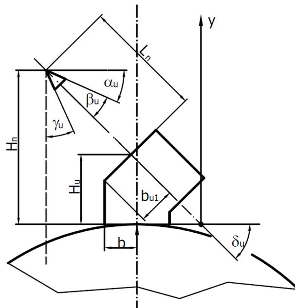
Figure 11. Diagram of the pick and holder on the cutting head.
