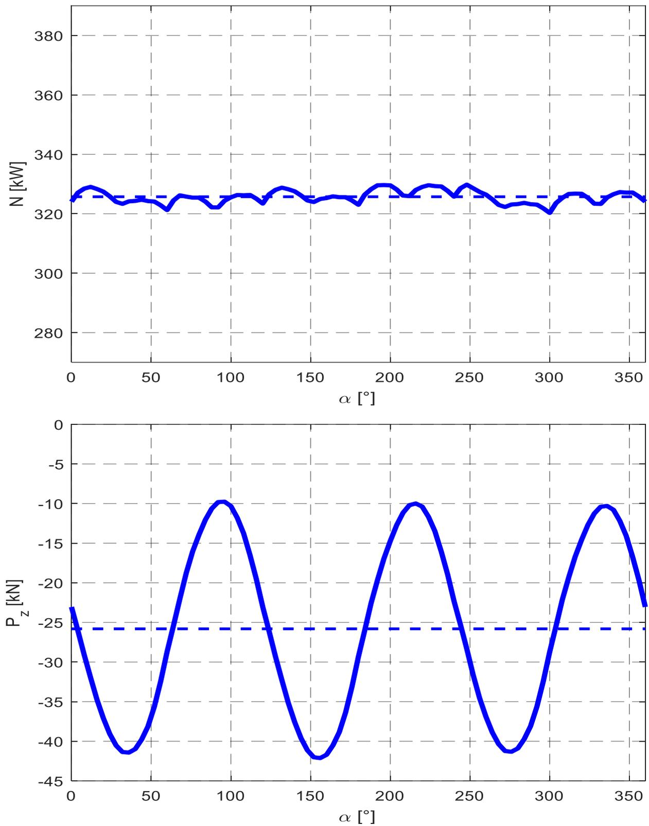
**Figure 16.** Waveform of the values of power  $N$  and cutting head impact force in the direction of shearer's advance  $P_z$  for pick arrangement 1d.
