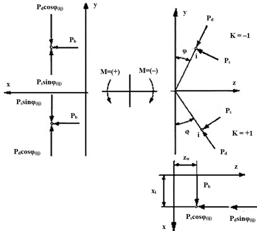
Figure 3. Diagram of the distribution of the components of cutting resistance forces on the  $i$ th pick [29].
