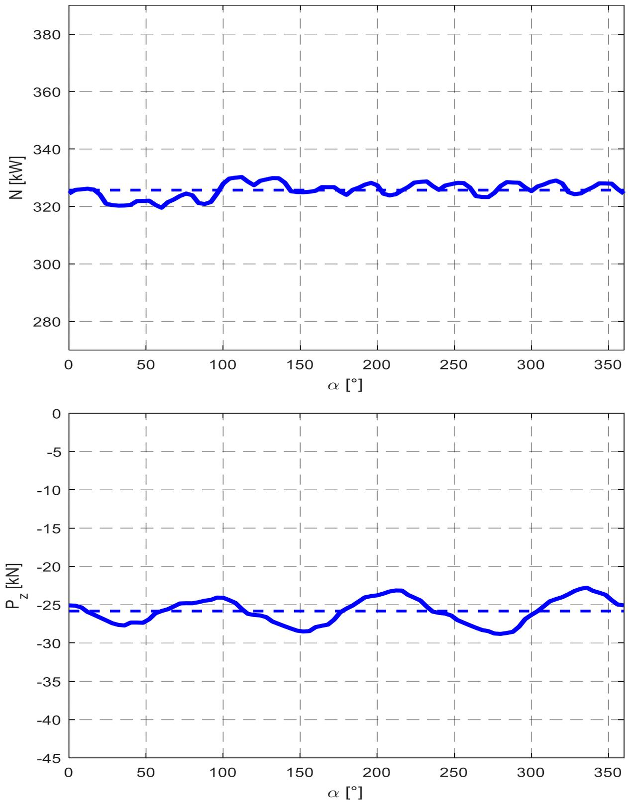
**Figure 15.** Waveform of the values of power  $N$  and cutting head impact force in the direction of shearer's advance  $P_z$  for pick arrangement 1c.
