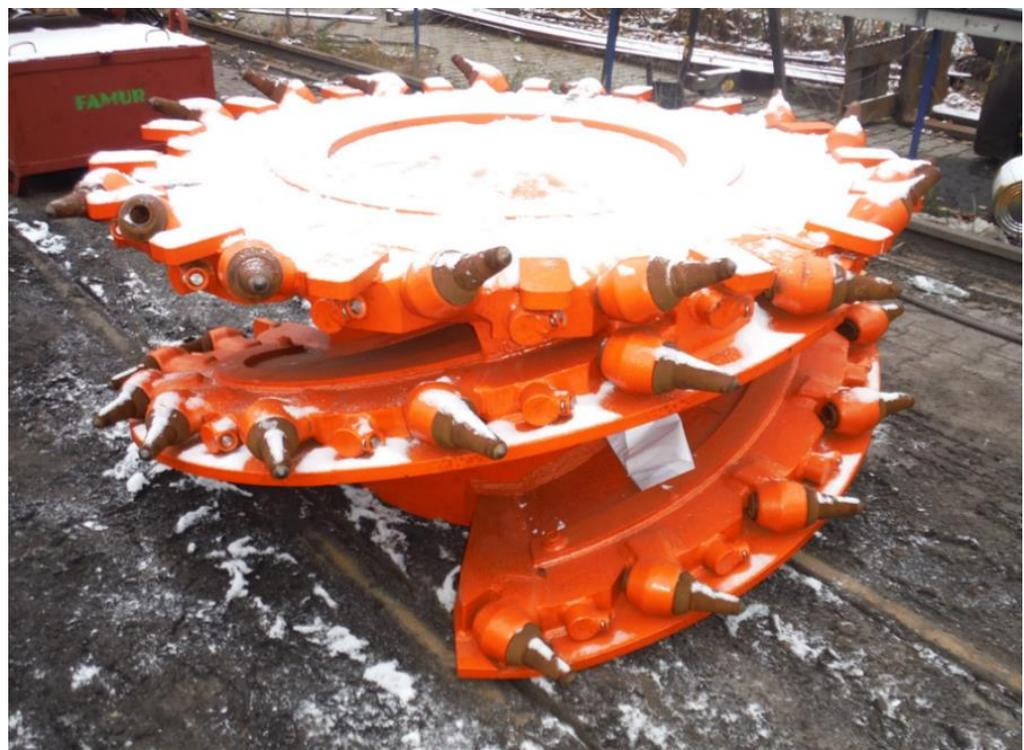
Figure 9. View of the analysed  $\varnothing 2030 \times 800$  cutting head.
