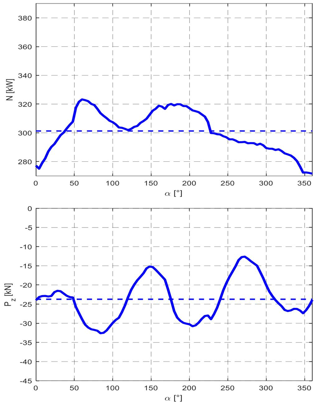
**Figure 12.** Waveform of the values of power  $N$  and cutting head impact force in the direction of shearer's advance  $P_z$  for pick arrangement 1.
