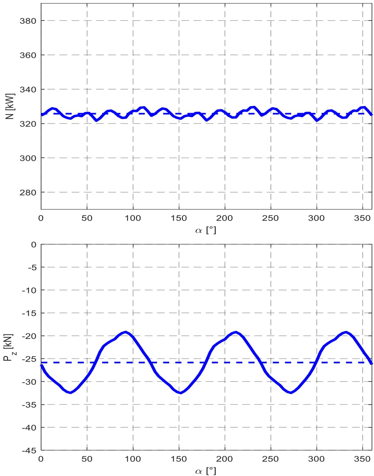
**Figure 14.** Waveform of the values of power  $N$  and cutting head impact force in the direction of shearer's advance  $P_z$  for pick arrangement 1b.
