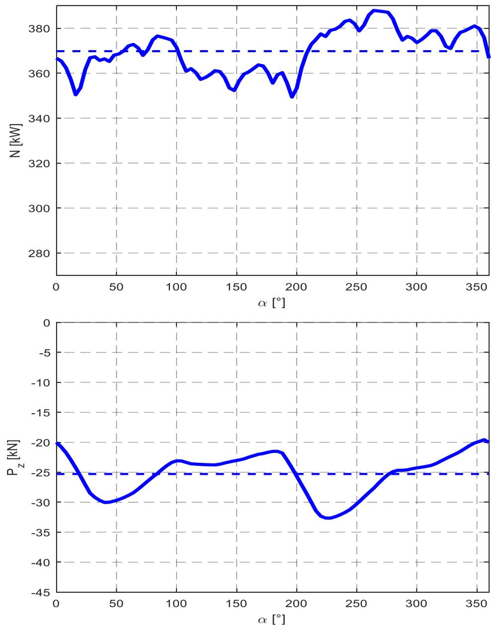
**Figure 17.** Waveform of the values of power  $N$  and cutting head impact force in the direction of shearer's advance  $P_z$  for pick arrangement 2.
