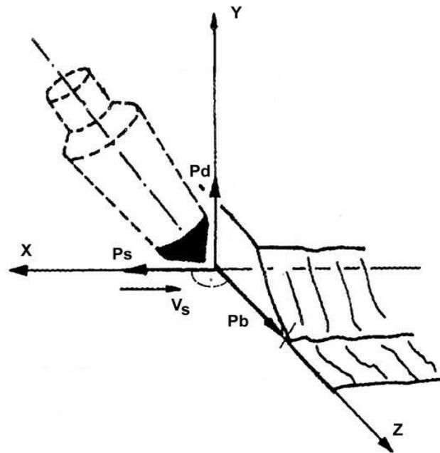
**Figure 2.** Forces acting on the pick during the cutting process:  $P_s$ —cutting force (tangent),  $P_d$ —pressure force (normal) and  $P_b$ —lateral force [28].
