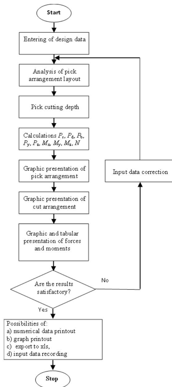
Figure 4. Block diagram of the program for designing the shearer cutting head [29].
