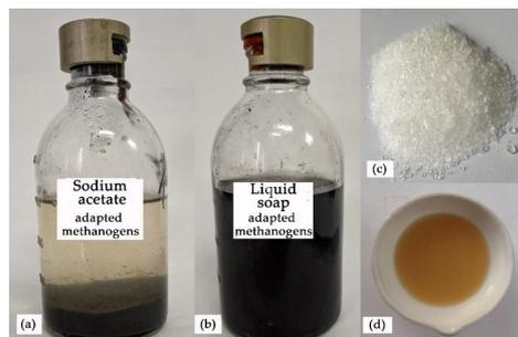
**Figure 1.** The methanogenic fermentation (13 days) of sodium acetate (a) and model soapstock (b), as well as sodium acetate crystals (c) and liquid soap (d), which were added to fermentation jars to prepare model stocks.
