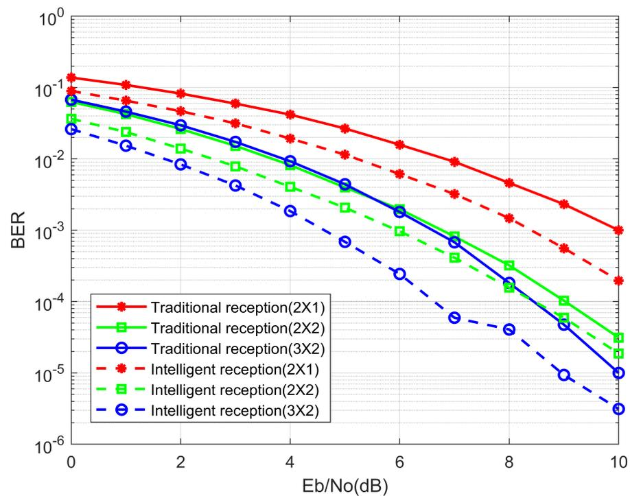
**Figure 11.** Comparison of information recovery capability for different antenna combinations.
