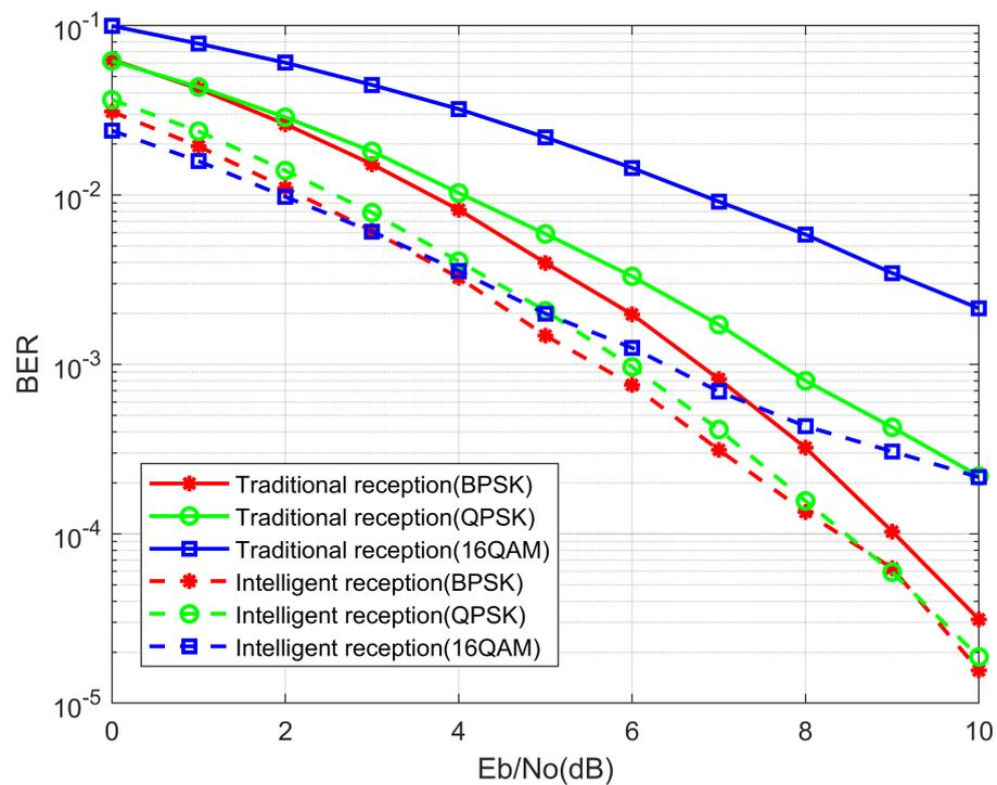
**Figure 10.** Comparison of information recovery capability for different modulation methods.
