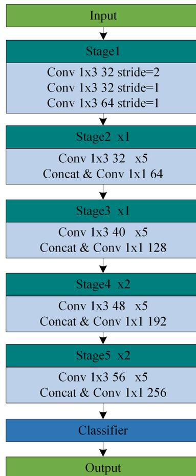
**Figure 7.** Network structure of mine intelligent receiver based on VOVNet.
