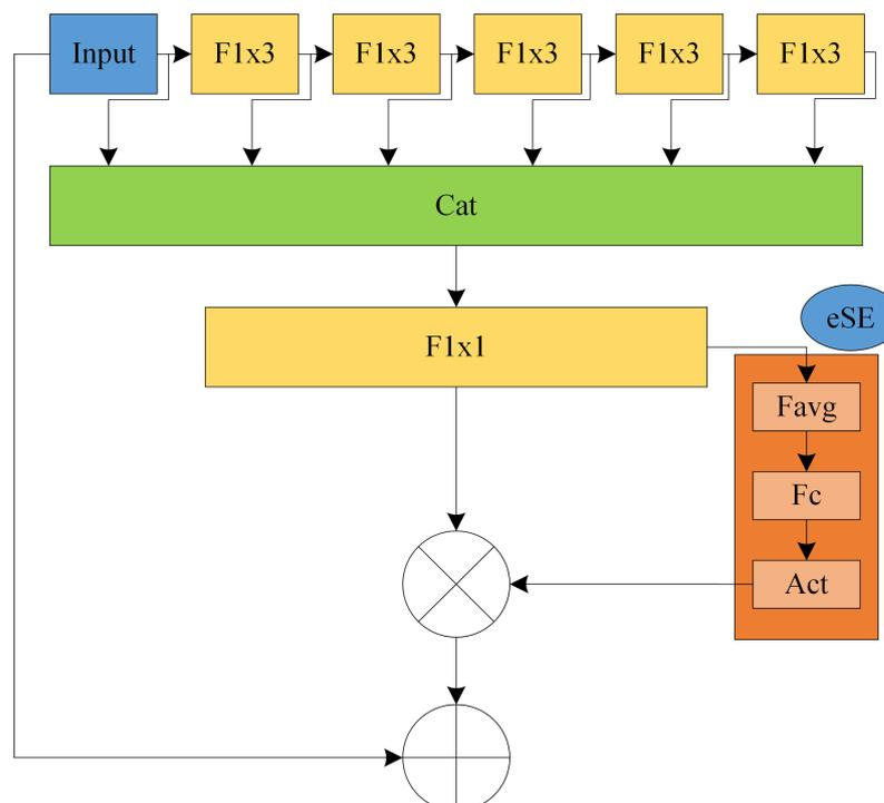
Figure 4. One-short aggregation module. F1x3 denotes the convolution operation with a convolution kernel of  $1 \times 3$ ; Cat denotes the feature map connected in the channel dimension; Favg denotes the global average pooling; Fc is the fully connected operation; Act is the h-sigmoid activation function;  $\otimes$  denotes element multiplication;  $+$  denotes element addition.
