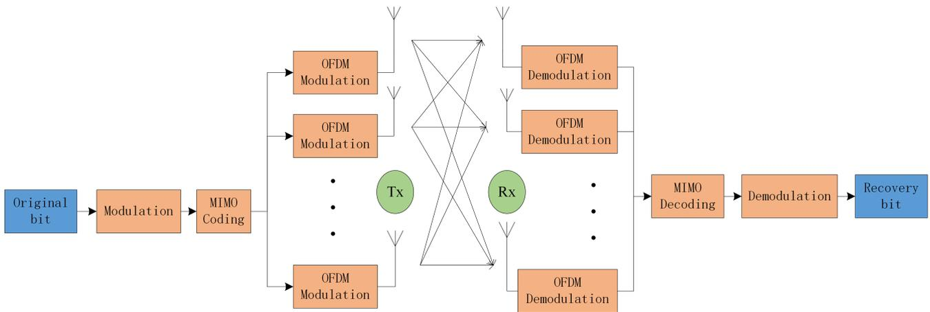
Figure 1. Conventional MIMO-OFDM system architecture.
