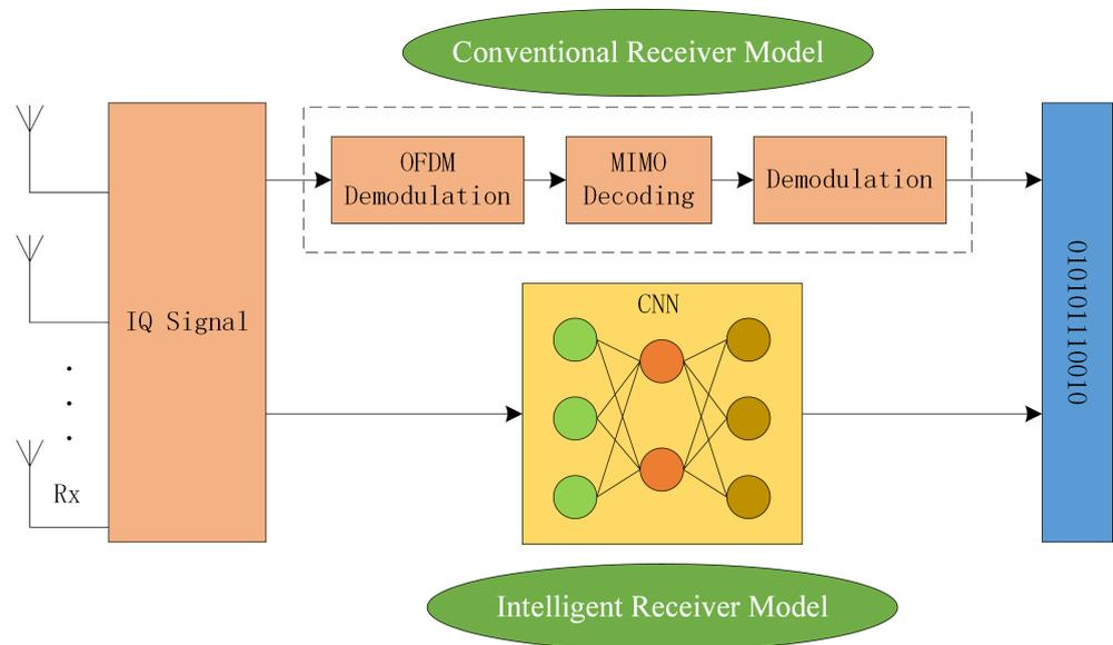
**Figure 6.** Structure comparison between traditional receiver and intelligent receiver.
