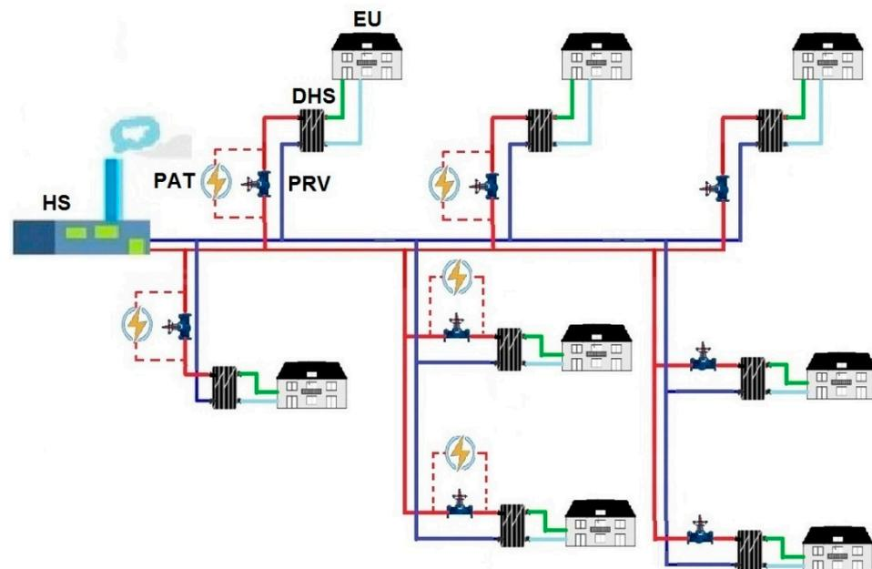
**Figure 10.** Typical micro hydro-turbine locations in a DHS: HS—heating station; PRV—pressure reducing valve; DHS—district heating substation; EU—end-user; PAT—pump as turbine.
