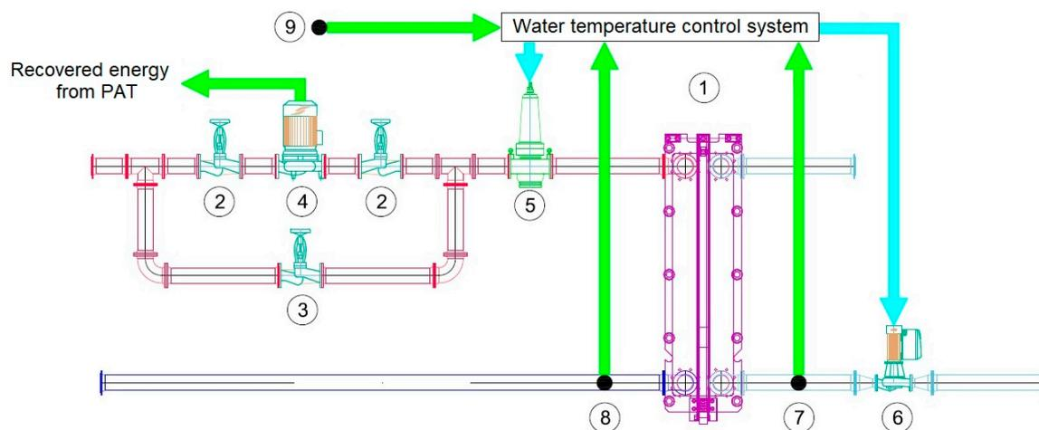
Figure 15. Pump as turbine (PAT) location scheme: 1—HX; 2—Control valve; 3—By-pass pipe; 4—PAT; 5—PRV; 6—Circulating pump; 7—Secondary circuit temperature sensor; 8—Primary circuit temperature sensor; 9—Outdoor temperature sensor.
