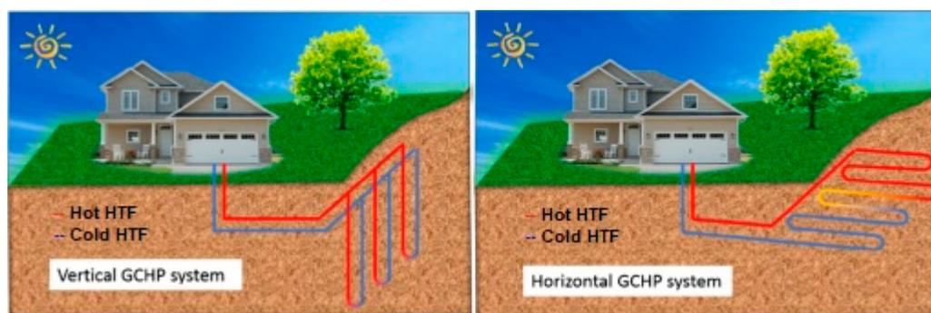
**Figure 8.** Horizontal and vertical ground heat exchanger (GHE) system configuration.
