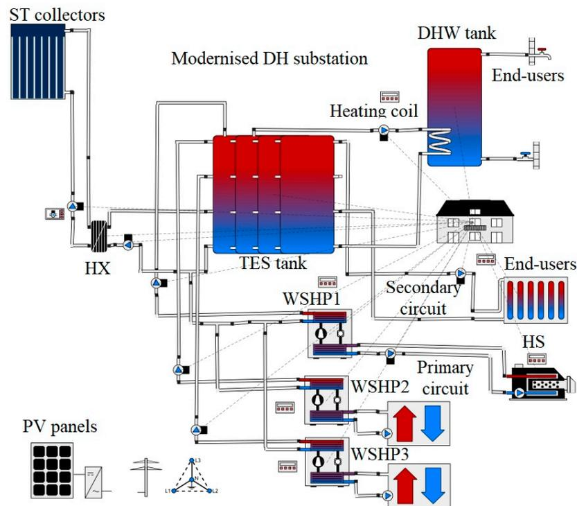
**Figure 12.** Schematic diagram of modernised “UMT” district heating (DH) substation.
