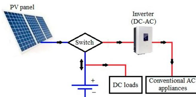
**Figure 5.** Diagram of a stand-alone photovoltaic (PV) system.
