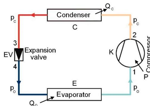
**Figure 7.** Scheme of a heat pump (HP) using vapour compression.
