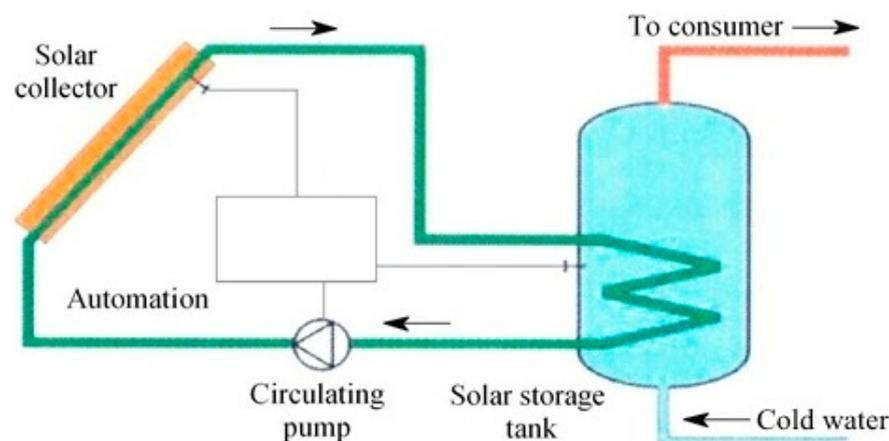
**Figure 4.** Conversion of solar energy to thermal energy.
