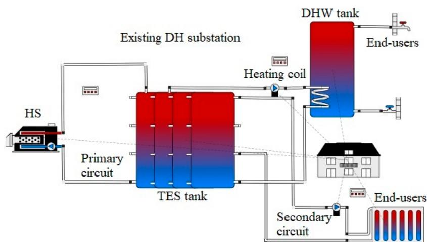
**Figure 11.** Schematic diagram of existing “UMT” district heating (DH) substation.
