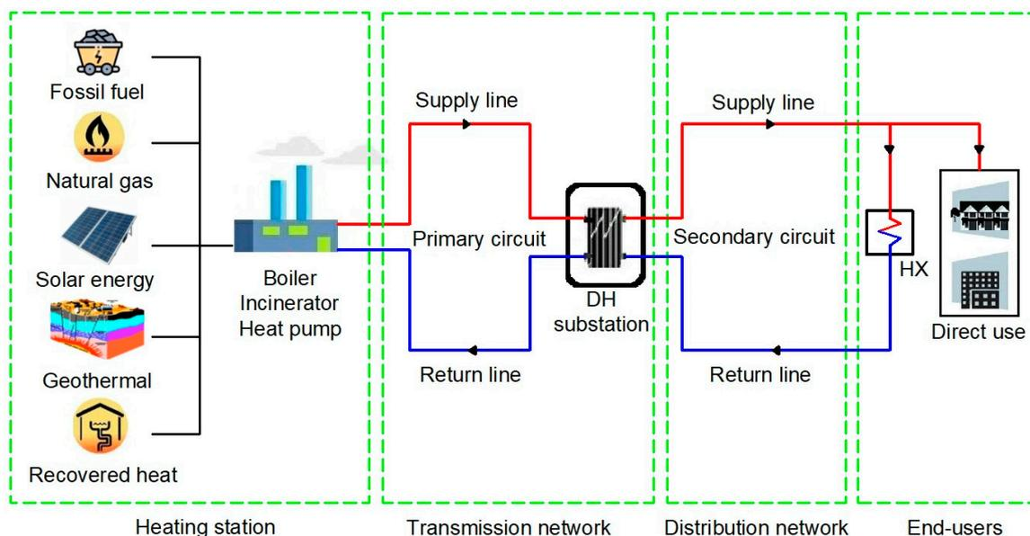
**Figure 1.** Essential district heating system components.
