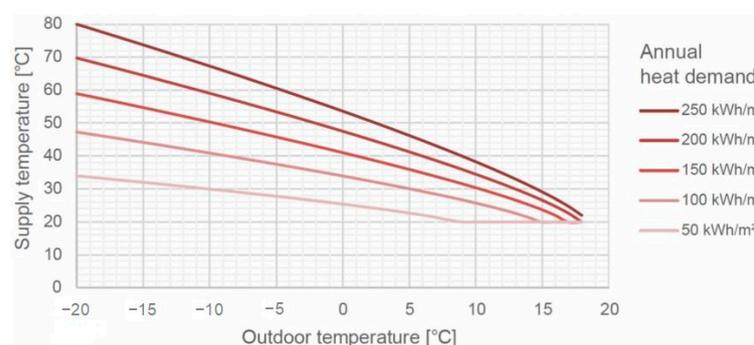
**Figure 2.** The necessary supply temperatures in a radiator [31].
