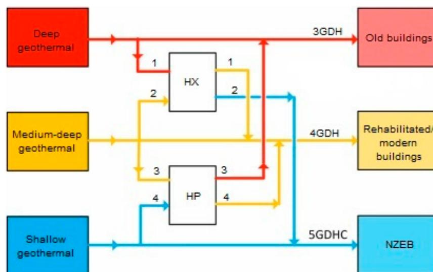
**Figure 9.** Scheme of the multi-depth geothermal system: 1-1—heat transfer from deep system to 4GDH; 2-2—heat transfer from medium-deep system to 5GDHC; 3-3—heat “upgrade” from medium-deep system to 3GDH; 4-4—heat “upgrade” from shallow system to 4GDH [31].
