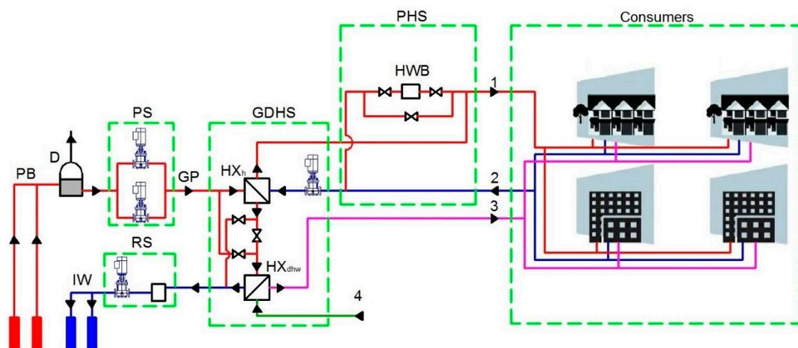
**Figure 6.** Schematic of a district heating system (DHS) utilising geothermal energy: PB—production borehole; D—degasser; PS—pumping station; GP—geothermal water pipe; GDHS—geothermal DH substation;  $HX_h$ —heat exchanger for heating;  $HX_{dhw}$ —heat exchanger for DHW; PHS—peak heating station; HWB—hot water boiler; IW—injection well; RS—reinjection station; 1, 2—pipes to and from heating installations; 3—DHW pipeline; 4—cold water pipes.
