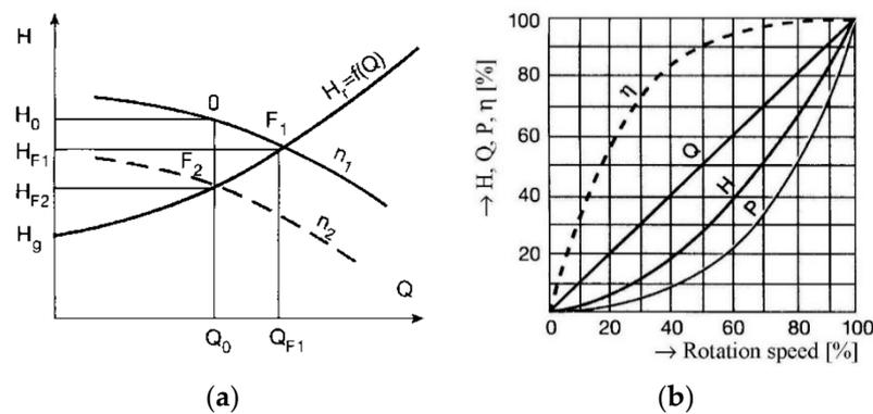
**Figure 18.** Quantitative regulation with variable-speed pumps (VSPs): (a) Discharge regulation by varying pump speed; (b) Centrifugal pump curves depending on rotation speed [123].
