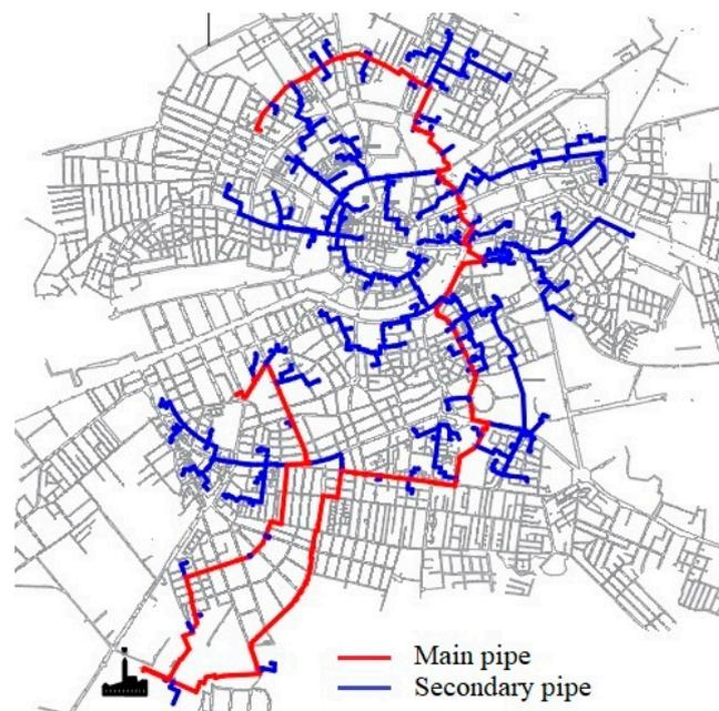
Figure 14. Scheme of the Timisoara heat transmission network.
