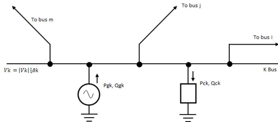
Figure 2. Detail of k-bus of Figure 1 generic grid.
