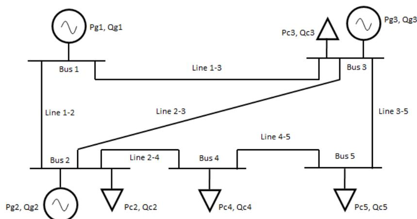
**Figure 1.** Typical scheme of a load flow power grid.
