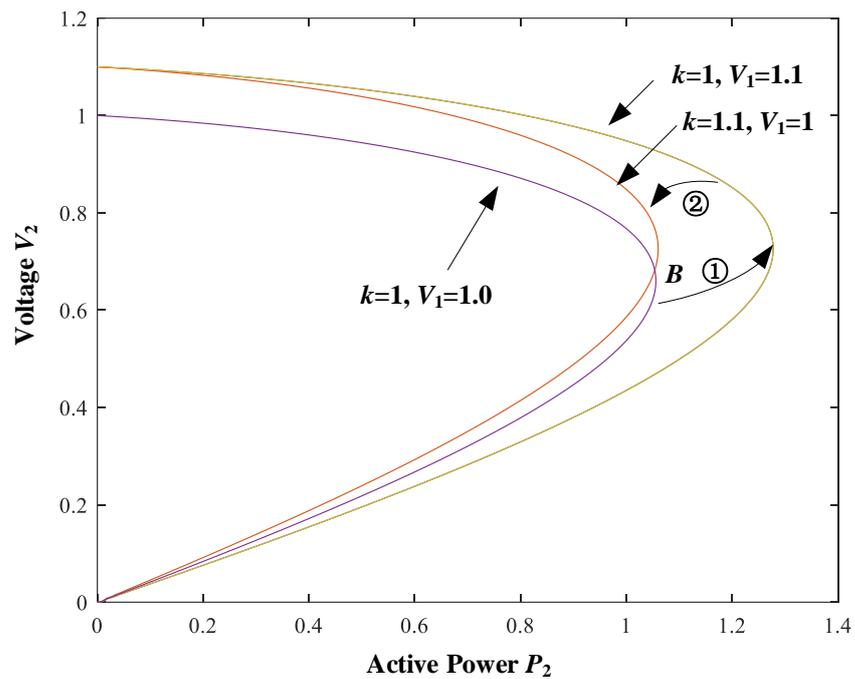
Figure 10. P-V curve of step and step-less voltage regulation with Flexible OLVR transformer. Point B is the intersection of two P-V curves.
