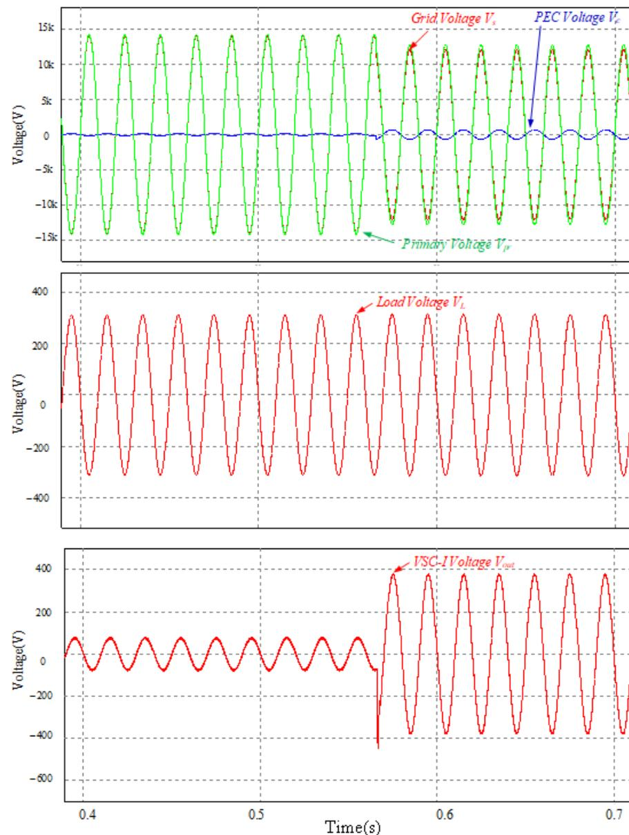
**Figure 14.** Voltage Waveforms during voltage regulation with Flexible OLVR.
