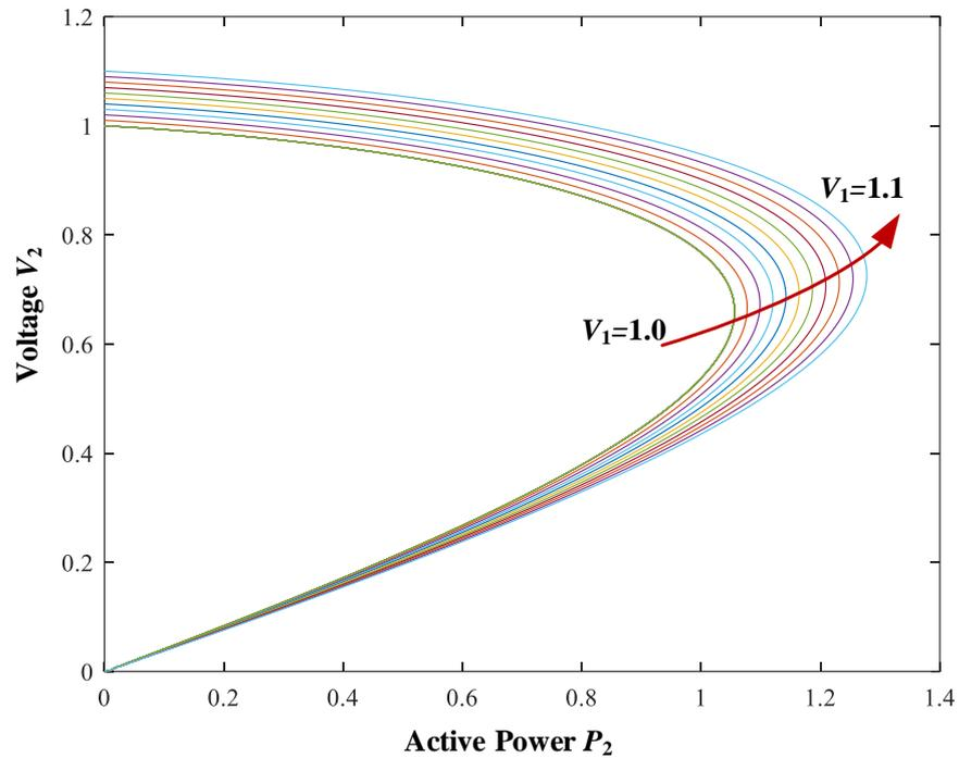
Figure 9. P-V curve of step-less voltage regulation process with Flexible OLVR transformer.
