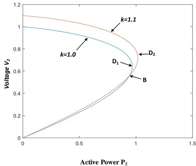
**Figure 6.** Positive voltage regulating effect of OLTC transformer. Point B is the intersection of the two P-V curves.
