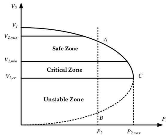
**Figure 4.** The load P-V curve of simple power system. Point A in is the stable operation point, and point B is the unstable point, Point C is the critical point of system.
