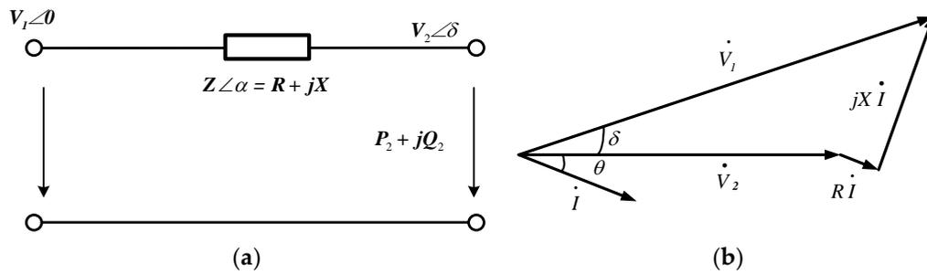
**Figure 3.** Equivalent circuit and phasor diagram of simple linear network in power system. (a) The Equivalent Circuit of simple linear network (b) The Phasor Diagram of simple linear network in power system.
