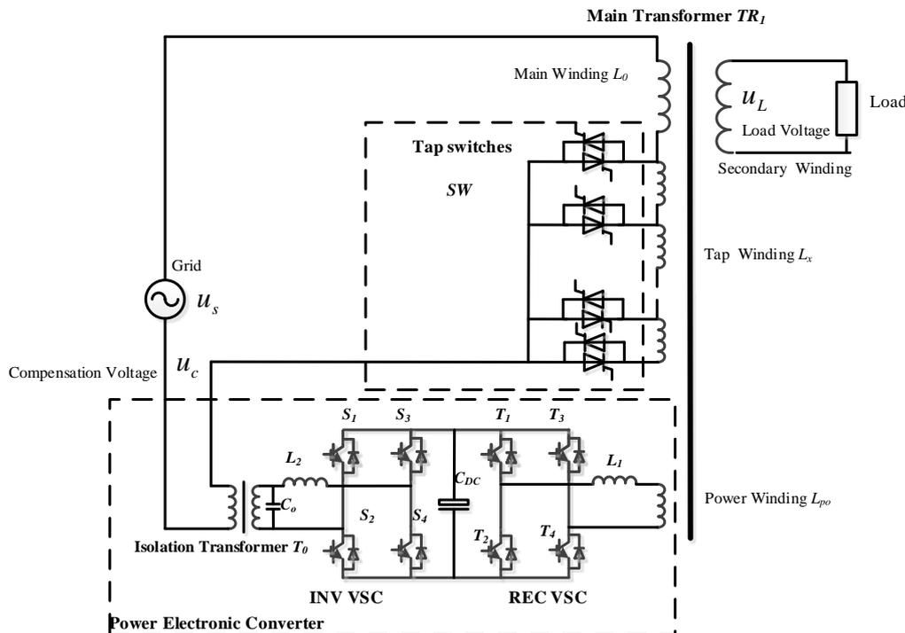
**Figure 1.** Single-phase topology structure of Flexible OLVR Transformer.
