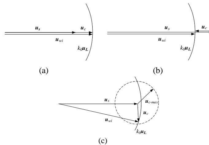
**Figure 2.** Voltage vector relationship of Flexible OLVR (a) The same direction compensation scheme (b) The reverse direction compensation scheme (c) Arbitrary direction compensation scheme.
