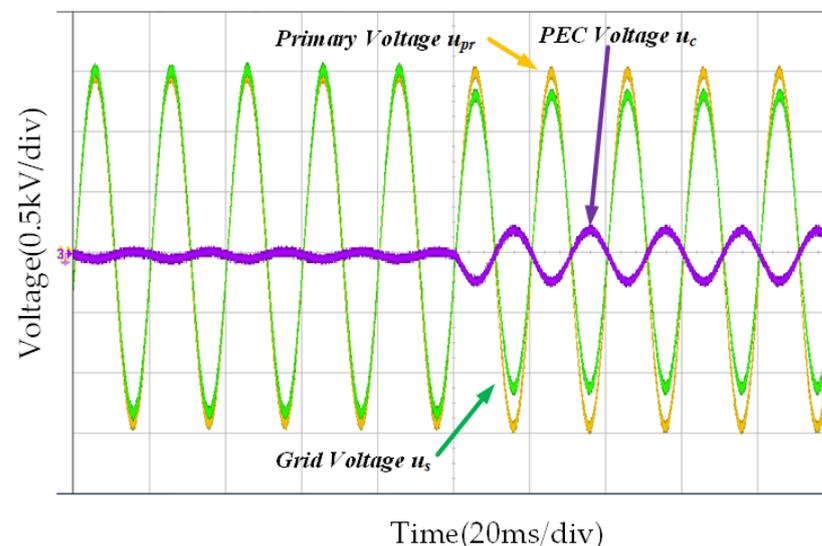
**Figure 15.** Waveform diagram of step-less voltage regulation with Flexible OLVR.
