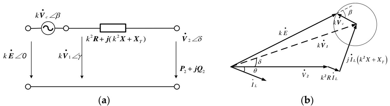
**Figure 8.** Equivalent circuit and phasor diagram of power system with Flexible OLVR transformer. (a) The equivalent circuit of power system with Flexible OLVR transformer; (b) The phasor diagram of power system with Flexible OLVR transformer.
