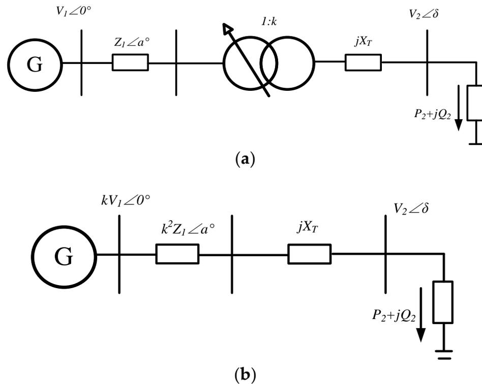
Figure 5. Simple system model and equivalent model with OLTC transformer. (a) The Simple Circuit of a power system with OLTC transformer (b) The Equivalent model with OLTC transformer.
