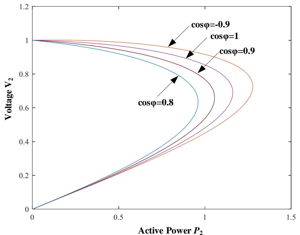
Figure 11. The P-V curves under different power factors.
