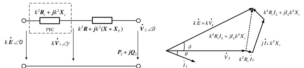
Figure 12. Equivalent circuit and phasor diagram of Flexible OLVR transformer based on controllable impedance equivalent.
