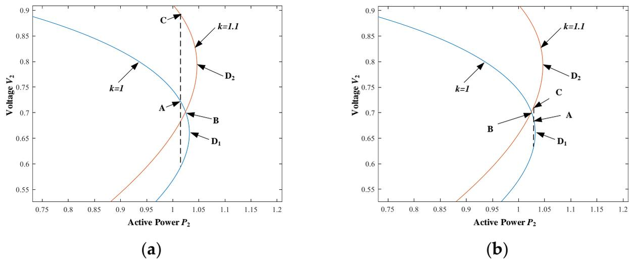
**Figure 7.** Deviation effect of critical operating point of OLTC transformer. (a) Positive adjustment; (b) Negative adjustment. Point A is initial operating point. Point B is the intersection of two P-V curves. Point C is operating point after OLTC action.
