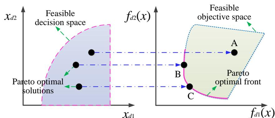
Figure 7. A specific case of the Pareto optimal solution.
