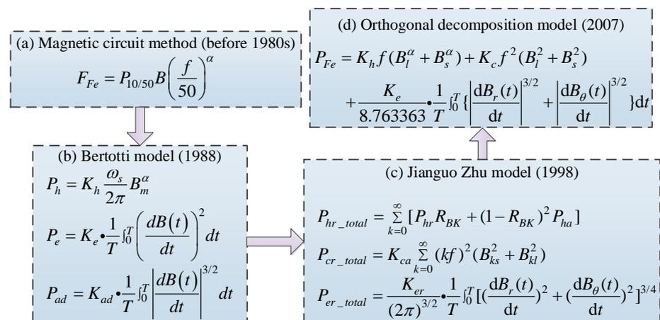
**Figure 1.** Development process of iron loss calculation models. Note:  $P_h$  is the hysteresis loss density,  $P_e$  the eddy current loss density and  $P_{ad}$  the additional loss density. The detailed explanations can also be found in the listed reference [22–24].
