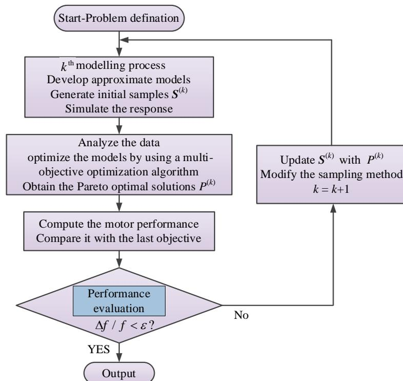
Figure 12. Flowchart for space reduction sequential optimization method.
