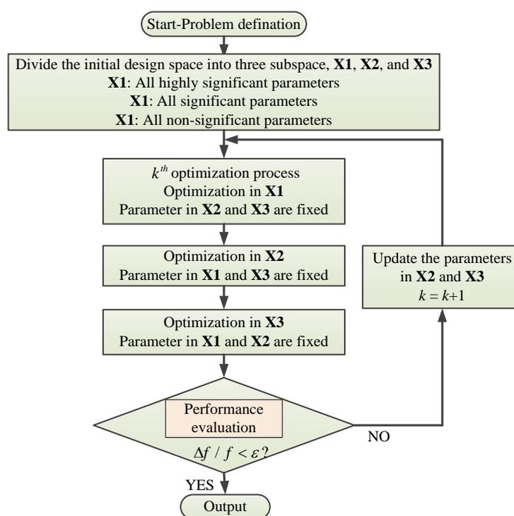
**Figure 10.** Flowchart for the multi-level optimization method.
