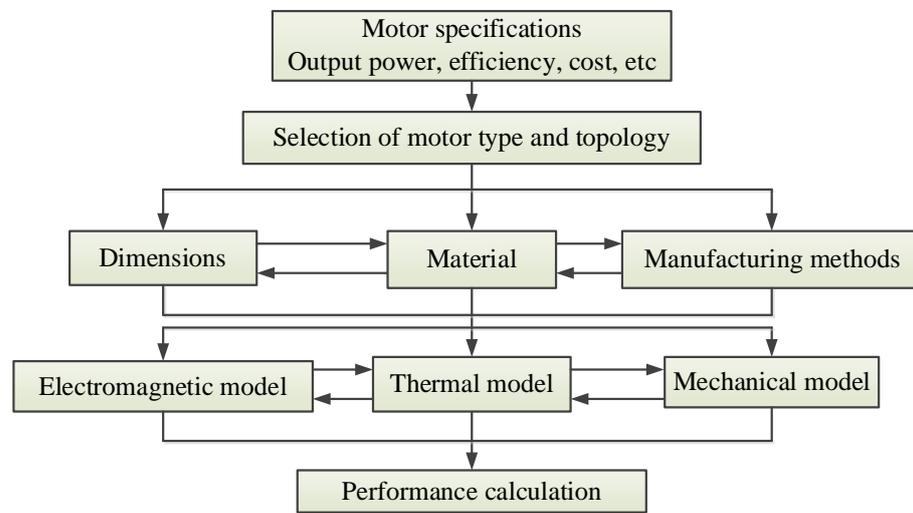
Figure 6. Design framework of HSPMMs and other electrical machines with multi-physics analysis.
