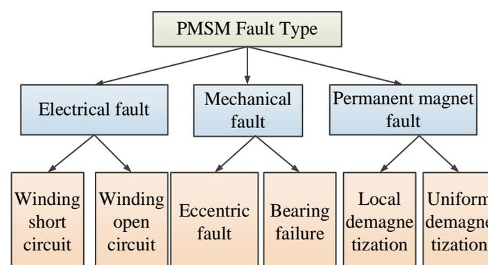
**Figure 5.** PMSM fault type.
