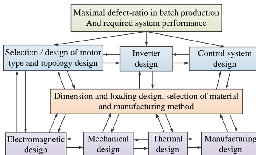
**Figure 9.** Robust design optimization framework of an electrical drive system.
