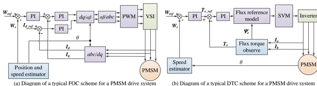
**Figure 2.** Control diagrams of typical FOC and DTC for PMSM drive systems. Note:  $I_d$  and  $I_q$  stand for the  $d$ - and  $q$ -axis currents, respectively.  $\psi_e$  is the flux,  $T_e$  the torque. For FOC, the  $d$ -axis current is set to zero for achieving the maximum torque per ampere. The current/torque loop and speed loop are set as feedback loops to keep the reference speed  $W_{ref}$  as well as to make a smaller  $d$ -axis reference current  $I_{d,ref}$ .
