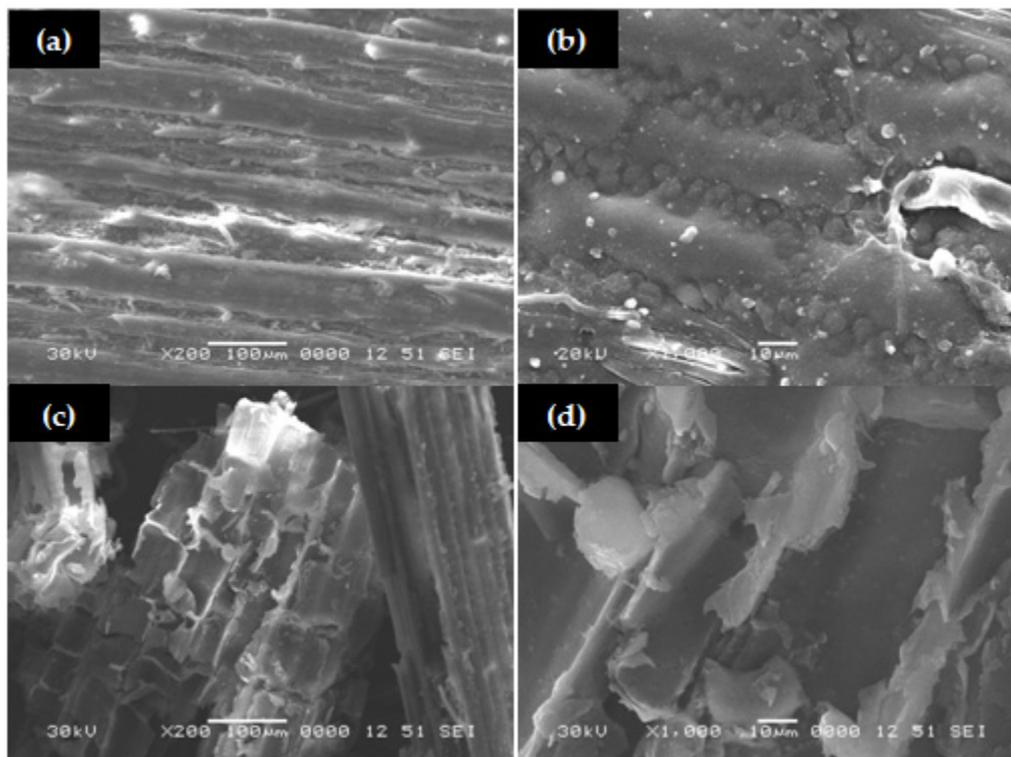
**Figure 6.** SEM images of (a,b) CS and (c,d) CSM.
