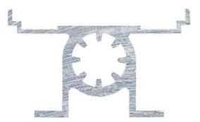
Figure 10. The cross-sectional view of CHAPS receiver tested in [92]. Reprinted with permission from Ref. [92]. 2005, Elsevier.
