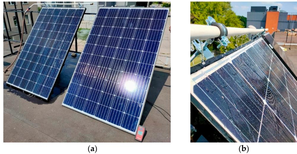
**Figure 5.** Experimental rig no. 2: (a) the general view of the experimental rig no. 2 with shown elements located on the roof, (b) a part of the water cooling system (header) installed on the tested 310 Wp PV panel.
