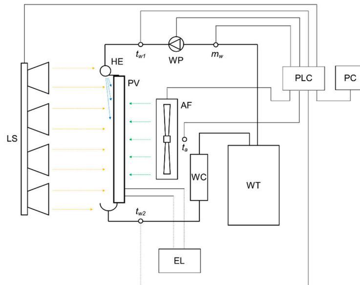
**Figure 3.** General scheme of the experimental rig (PV: PV panel, LS: light source, AF: air fan, WT: water tank, HE: header, WP: water pump, WC: water cooler, EL: electronic load, PLC: programmable logic controller, PC: computer,  $t_{w1}$ ,  $t_{w2}$ ,  $t_{air}$ : temperature sensors,  $m_w$ : water flowmeter).
