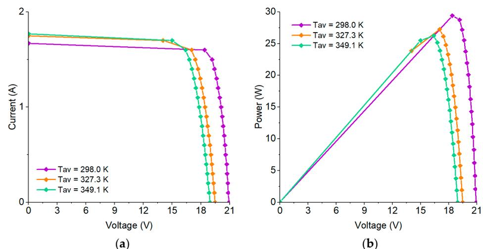
**Figure 7.** Variations in the performance of the 50 Wp PV panel depend on its temperature (without any cooling system): I-V characteristic (a) and P-V characteristic (b).
