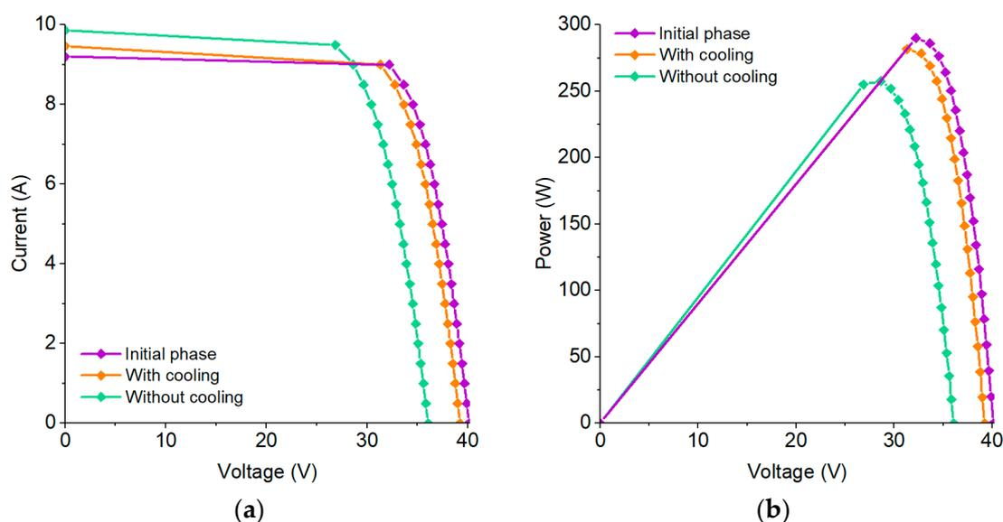
**Figure 13.** Variations in the performance of the 310 Wp PV panel depending on its temperature: I-V characteristic (**a**) and P-V characteristic (**b**).
