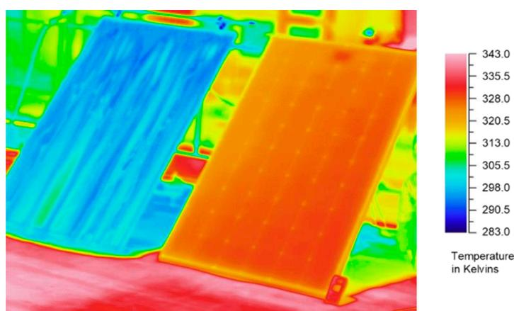
**Figure 12.** Thermal images show the temperature on the front surface of the tested 310 Wp PV panel without cooling (**right panel**), and with a water cooling system (**left panel**).
