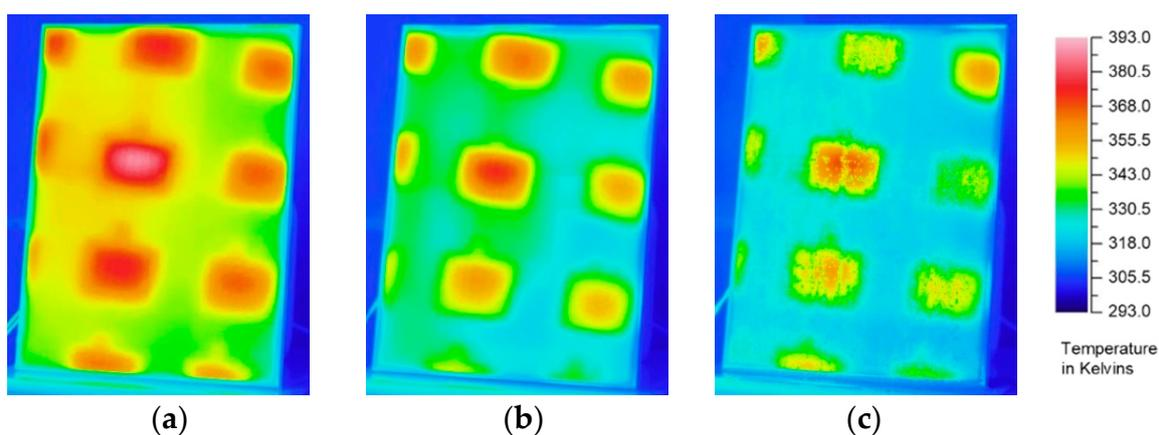
**Figure 8.** Temperature distribution on the front side of the 50 Wp PV panel after 15 min of the experiment: (a) without cooling, (b) with air cooling, (c) with a water cooling system (visible areas with higher temperature result from the configuration of the light source).
