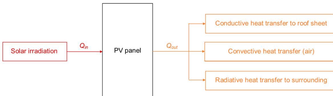
**Figure 1.** Thermal balance of the PV panels.
