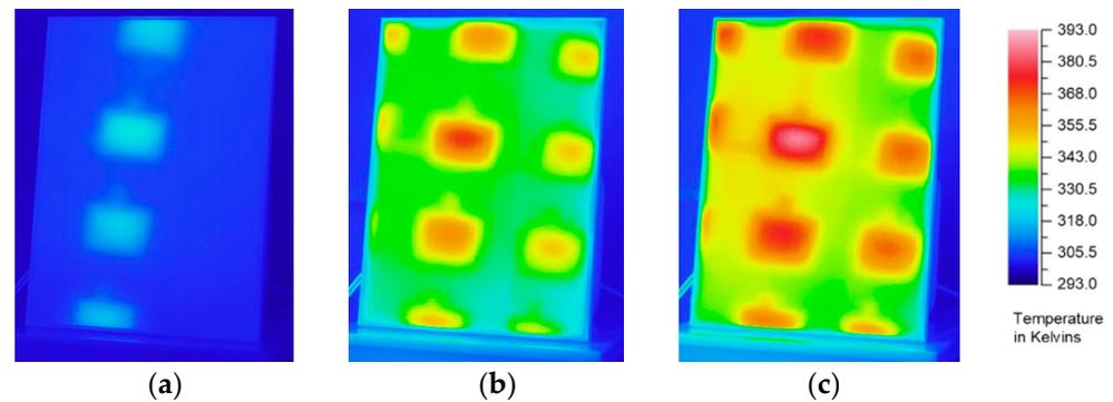
**Figure 6.** Temperature distribution on the front side of the 50 Wp PV panel during experiment: (a) beginning of the experiment, (b) after 7.5 min, (c) after 15 min (visible areas with higher temperatures are a result of the configuration of the light source).
