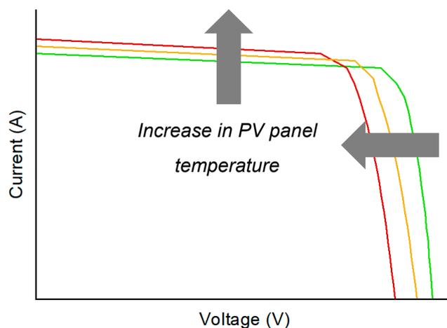
**Figure 2.** The impact of temperature on the operating characteristic of PV panels.
