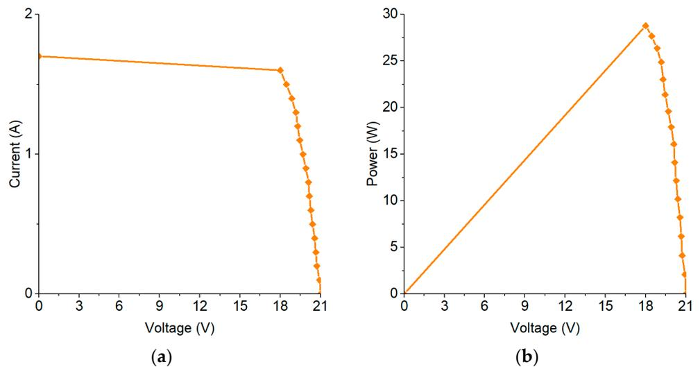
**Figure 11.** Variations in the performance of the 50 Wp PV panel depend on its temperature (when the prototype of water cooling system was installed and used): I-V characteristic (a) and P-V characteristic (b).
