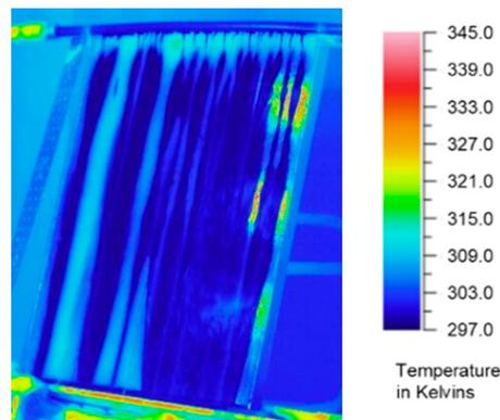
**Figure 10.** Temperature distribution on the front side of the 50 Wp PV panel after 15 min of the experiment (when dedicated water cooling system was used).
