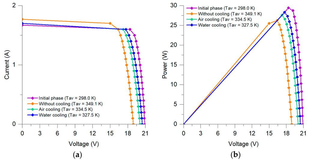
**Figure 9.** Variations in the performance of the 50 Wp PV panel depend on its temperature (resulted from the cooling method used): I-V characteristic (a) and P-V characteristic (b).
