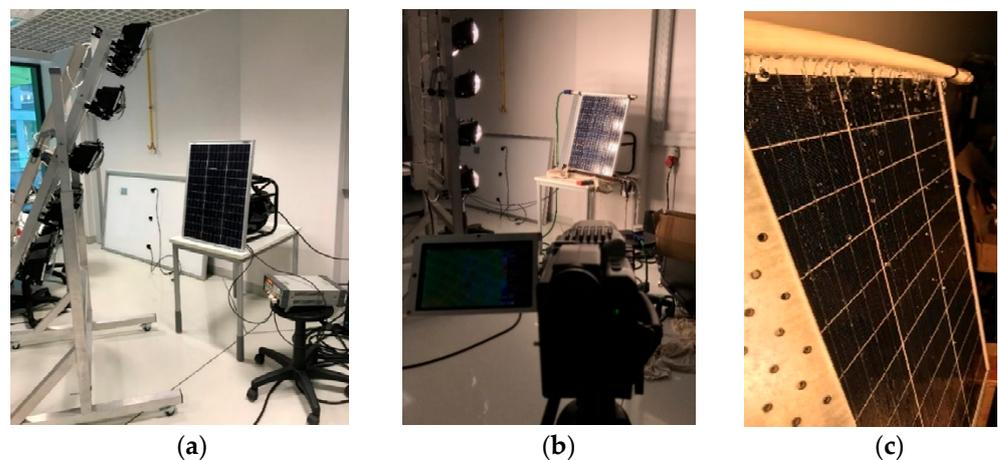
**Figure 4.** Experimental rig no. 1: (a) general view of the experimental rig no. 1, (b) experimental rig during tests with an infrared camera, (c) a part of the water cooling system (header) installed on the tested 50 Wp PV panel.
