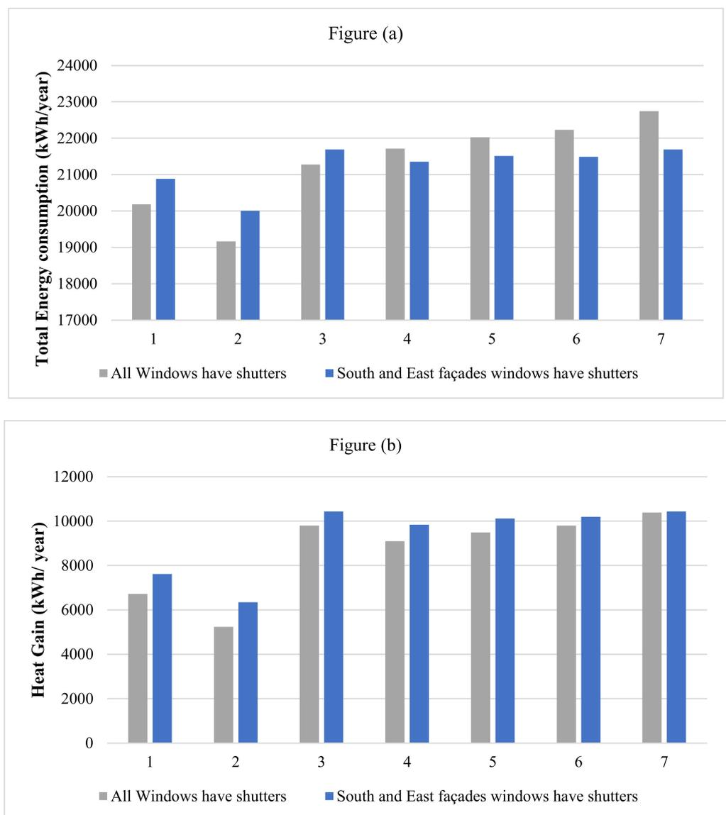
Figure 11. The total energy consumption (a) and heat addition (b) for the first case scenario: all windows have shutters and second case scenario: south and east windows have shutters with seven different windows shutter mechanism.
