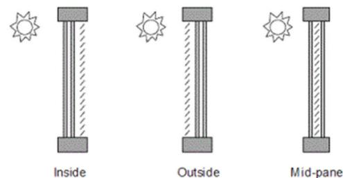
**Figure 2.** The positioning of windows shading devices (From DesignBuilder).
