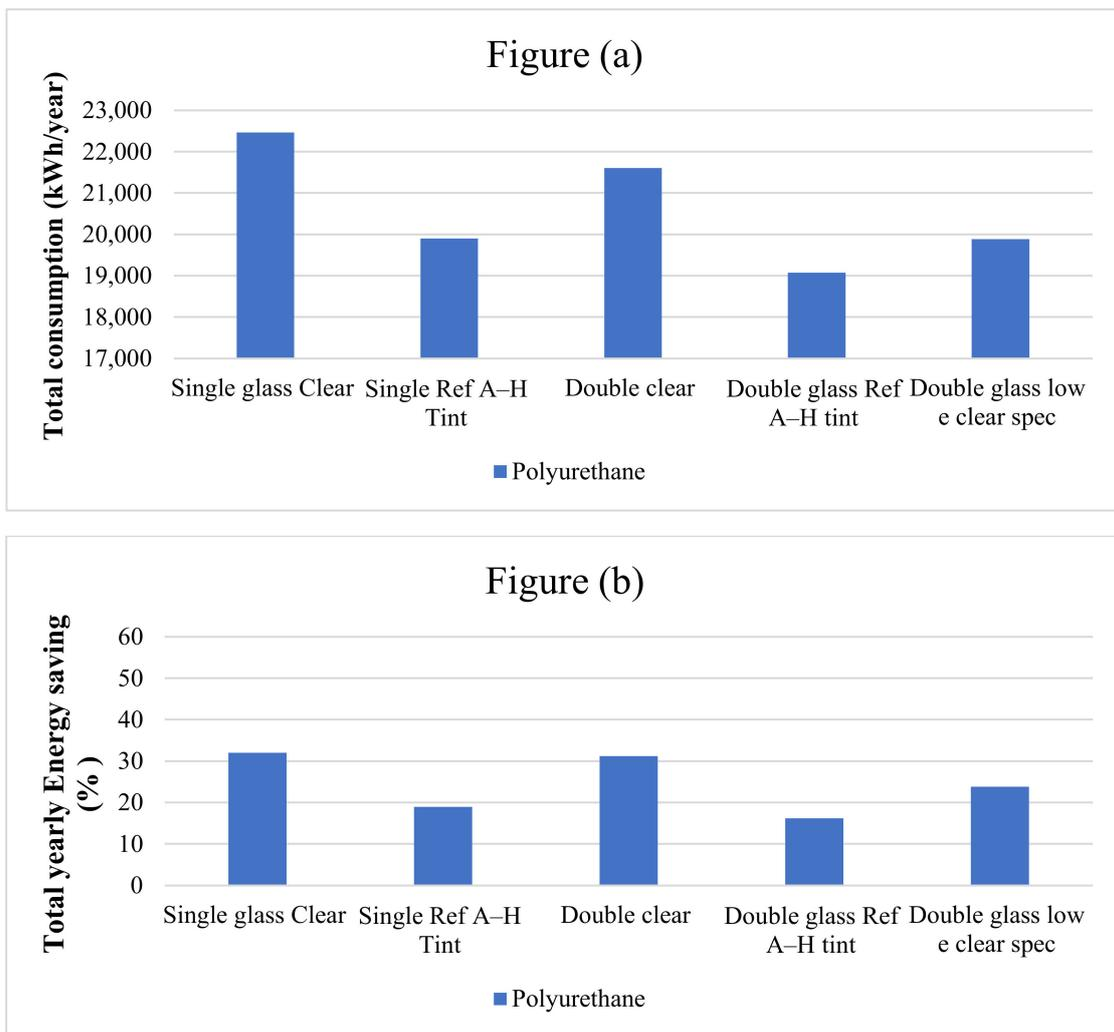
Figure 5. Effect of window shutters for different glass type on the total energy consumption of the building (a) and the correlated yearly total energy saving (b).
