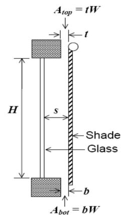
**Figure 3.** Configurations of external windows shading devices applied in the study (From DesignBuilder).
