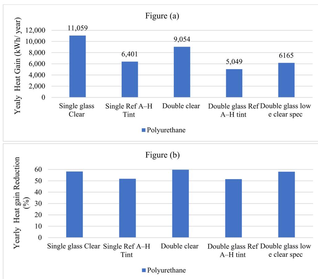
**Figure 4.** Effect of window shutters for different glass type on heat gain (a) and the correlated yearly heat reduction (b).
