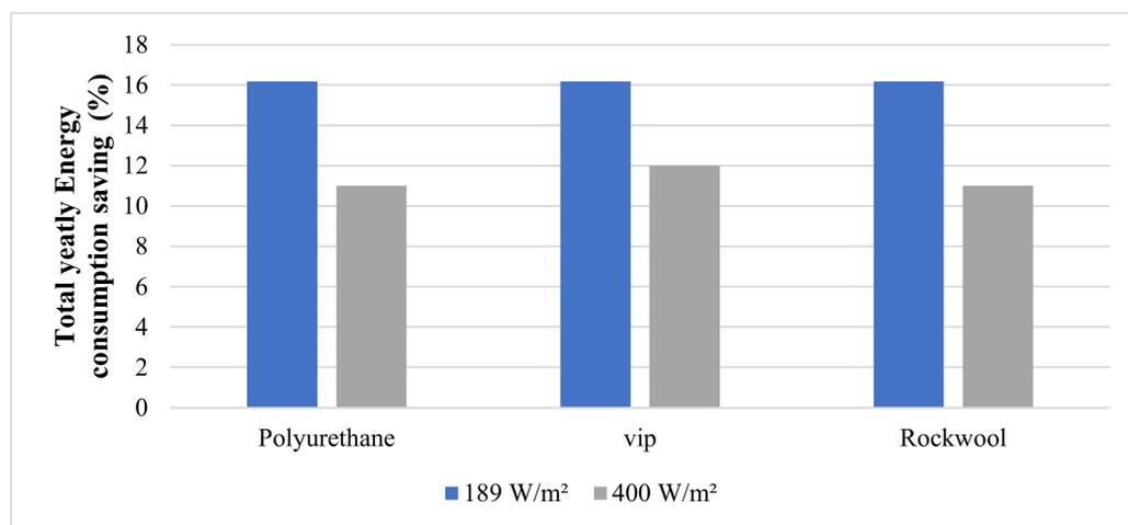
**Figure 9.** Yearly reduction in the total energy consumption of the building applying different types of window glass integrating three types of window shutters' insulations for different solar intensities.
