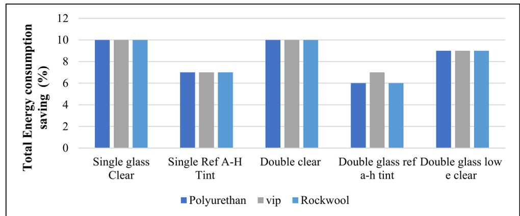
Figure 10. Total energy saving for different types of window glass with the three types of window shutters' insulations applying the glare with index 18.
