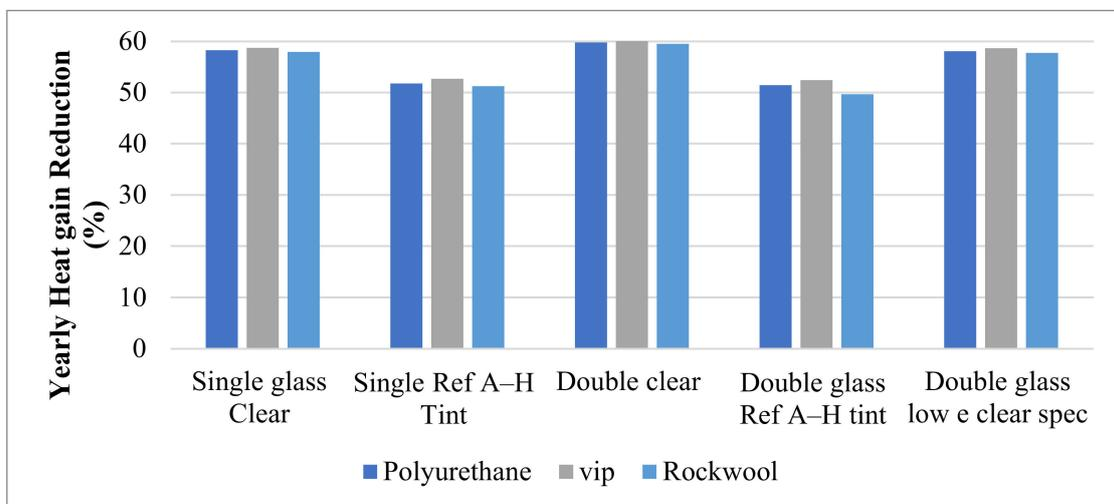
Figure 6. Yearly reduction in the total heat gain through different types of window glass applying three types of window shutters' insulations.
