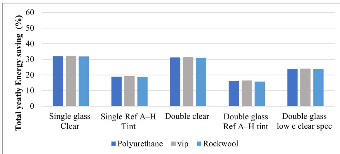
**Figure 7.** Yearly reduction in the total energy consumption of the building applying different types of window glass integrating three types of window shutters' insulations.
