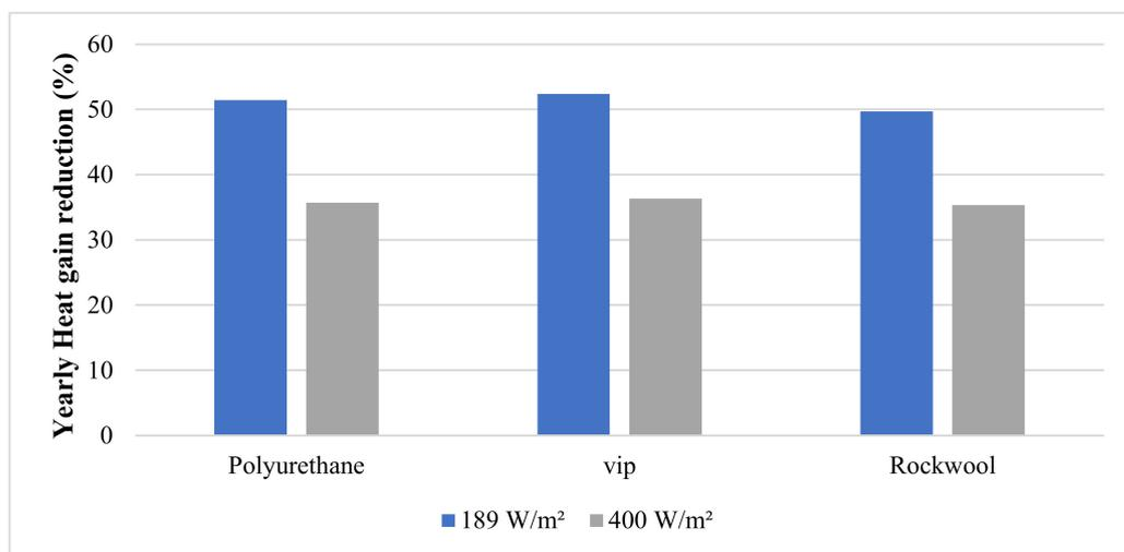
**Figure 8.** Yearly reduction in the heat gain of the building applying different types of window glass integrating three types of window shutters' insulations for different solar intensities.
