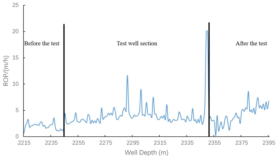
**Figure 4.** Drilling records of WWY1 section (2244–2350 m) using drill string absorption & hydraulic supercharging & speed-up technology.
