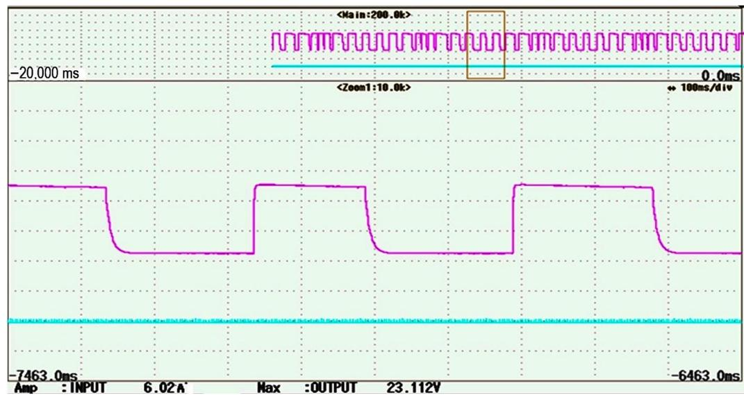
Figure 21. Input current and voltage waveforms under reverse mode of operation.
