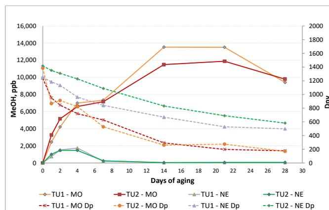
**Figure 3.** Change of methanol concentration and  $DP_v$  during aging experiment (TU papers in mineral and natural ester oil at 140 °C).
