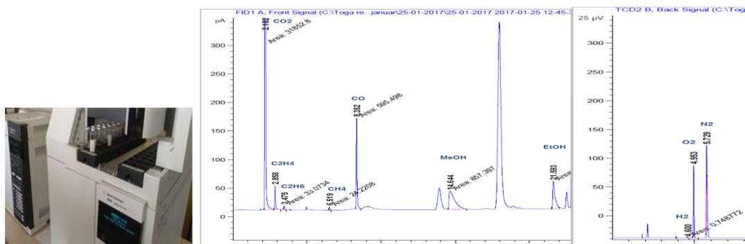
Figure 1. TOGA GC FID analyzer (left) and chromatogram of DGA and LMA (right).
