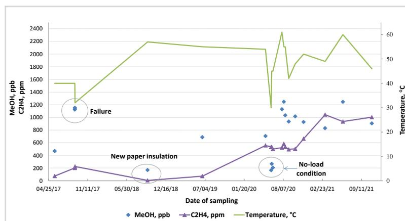
Figure 6. Change in methanol and ethylene concentrations before and after the failure.
