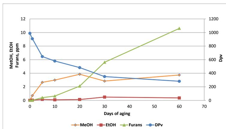
**Figure 2.** Change of methanol, ethanol and furan concentration and DP<sub>v</sub> during aging experiment II at 120 °C.
