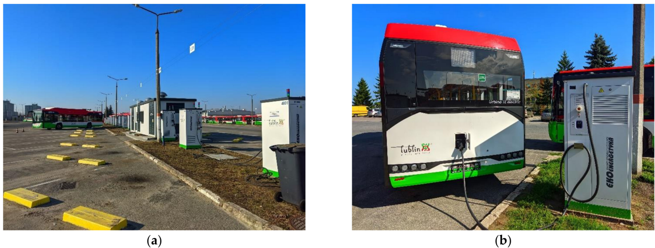
Figure 1. The view of (a) the bus depot and dedicated substation at the Grygowa Street; (b) Solaris Urbino Electric 12 electric bus being charged with the fast charger.
