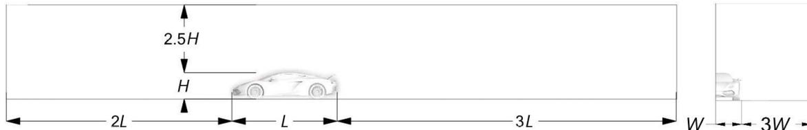
**Figure 20.** Size of the computational domain with length  $L = 4.6$  m height  $H = 1.1$  m and width  $W = 1.1$  m.
