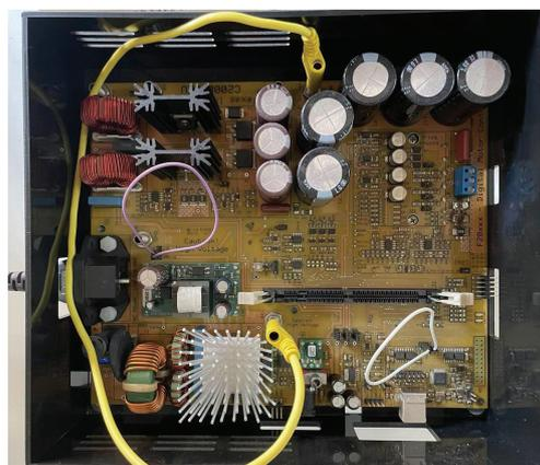
**Figure 24.** TI HVMTRPFCKIT inverter.
