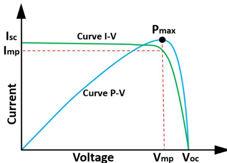
**Figure 2.** I-V and P-V curves of a SPV panel (adapted with permission from Ref. [108] Copyright 2015, Kumar, P., et al.).
