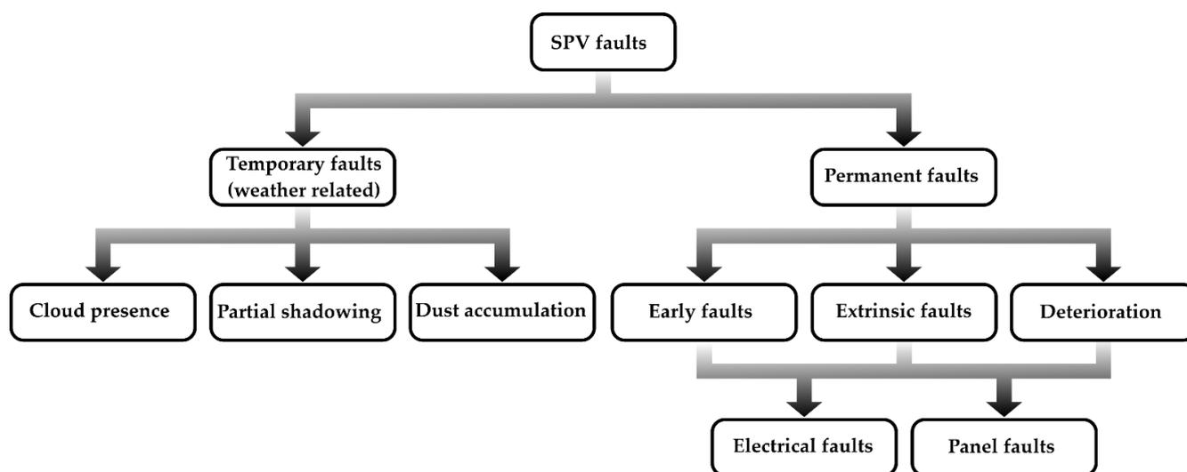
**Figure 1.** Type of faults in SPV systems.
