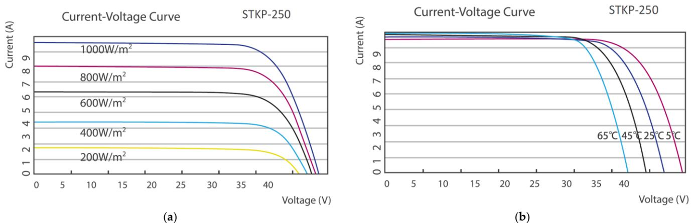
**Figure 3.** I-V curves of an SPV panel for (a) different solar radiation conditions and (b) different temperature conditions (adapted with permission from Ref. [107] Copyright 2022, Solar Electric London UK).
