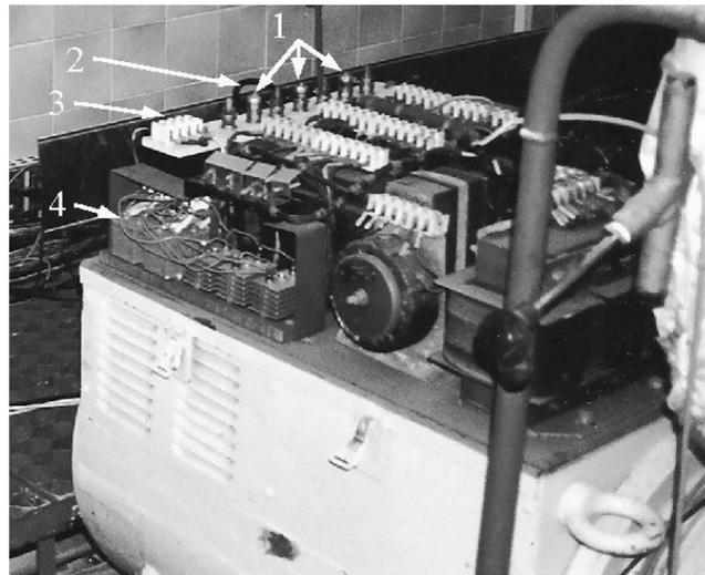
**Figure 3.** The WS 60 N voltage regulator with the current and voltage measuring points marked.
