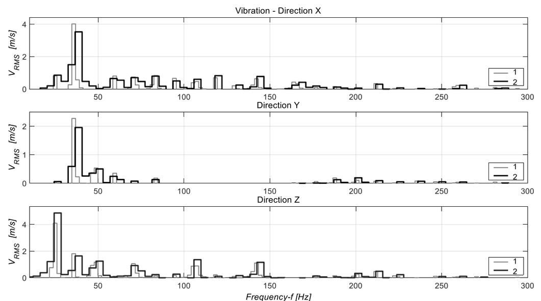
**Figure 9.** The fault at point 4 where the foundation frame is mounted to the ground—spectrum of the effective vibration velocity value: 1—rated signal; 2—signal during the breakdown.
