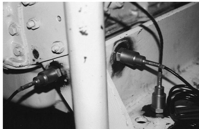
**Figure 4.** A view of the mounting point of the accelerometers on the foundation frame used for measuring vibrations in three directions.
