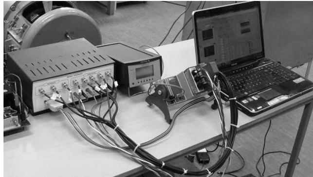
Figure 5. Modular computer subsystem used for measuring diagnostic parameters.
