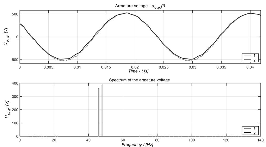
**Figure 8.** Phase-to-phase voltage  $U_{V-W}(t)$ : fault no. 3 to the governor speed controller. Load rate 100%  $P_n$ : 1, rated signal; 2, signal during the breakdown.
