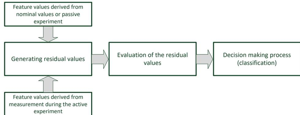
**Figure 7.** Diagram of the process of generating the residual values.
