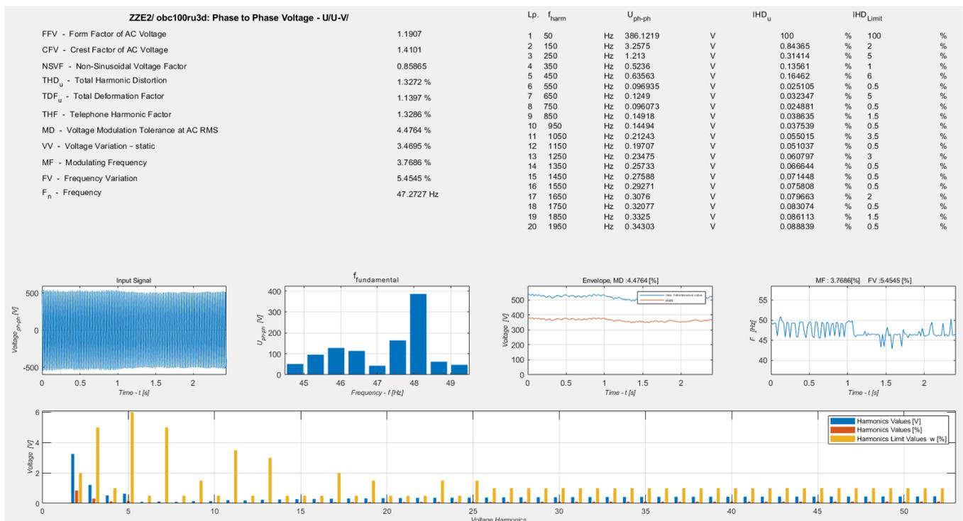
Figure 6. The MATLAB user interface of the ELPAR application: a set of analyses for synchronous generator armature voltages.
