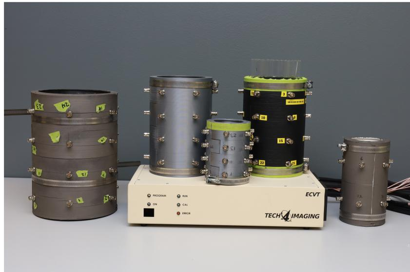
**Figure 2.** Data acquisition system and several cylindrical ECVT sensors of various sizes and with different numbers of electrode channels.
