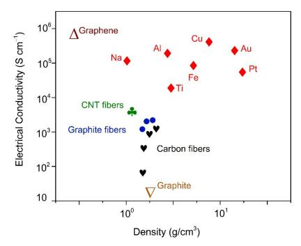
Figure 6. Electrical conductivity of materials [67] (p. 17).
