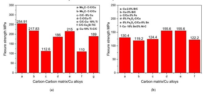
**Figure 5.** (a) Flexural strength of C/C matrix-Cu composites (a: [44]; b: [43]; c: [55]; d: [38]; e: [39]; f: [45]; g: [40]); (b) carbon matrix/Cu composites (a: [47]; b: [48]; c: [49]; d: [52]; e: [53]; f: [54]).
