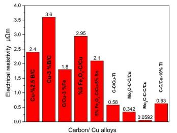
Figure 7. Electrical resistivity of carbon/Cu composites.
