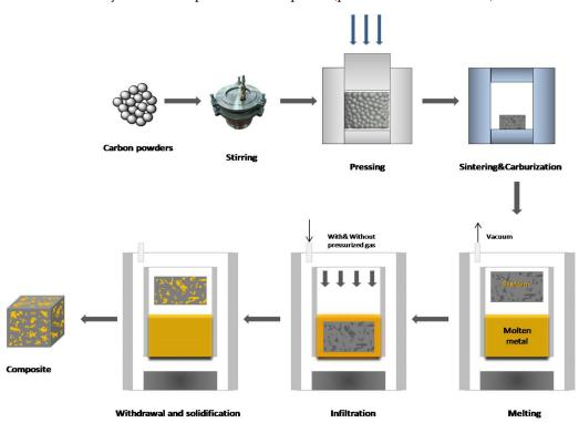
Figure 1. Gas infiltration process.
