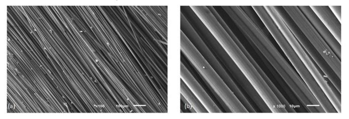
**Figure 2.** SEM images of long carbon fibers K1100 typically used for the preparation of carbon preform: (a)  $100 \times$  magnification image; (b)  $1000 \times$  magnification image (IMMS SAS).
