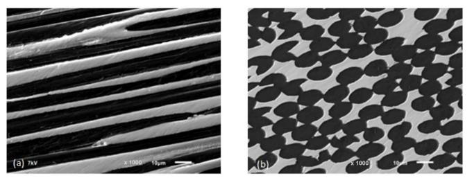
**Figure 3.** SEM microstructure of prepared Cf/Cu composites: (**a**) longitudinal to fibers; (**b**) perpendicular to fibers (IMMM SAS).
