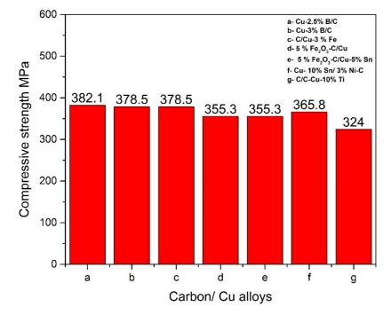
Figure 4. Compressive strength of composites (a: [47]; b: [48]; c: [49]; d: [52]; e: [53]; f: [54]; g: [39]).
