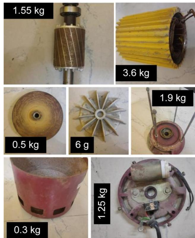
**Figure 2.** Weights of various parts of the motor.
