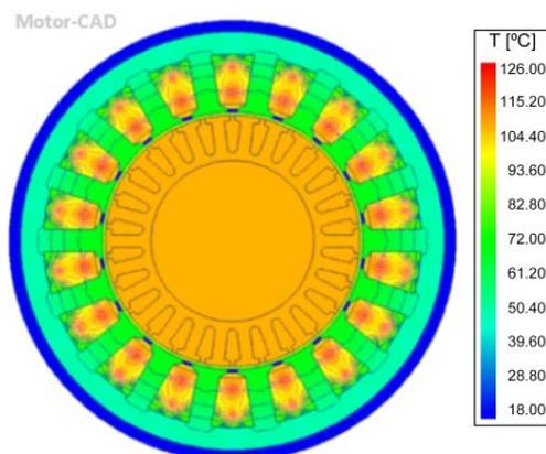
**Figure 14.** Radial view of PA6GF30 casing electric motor (water-cooled after FEM analysis).
