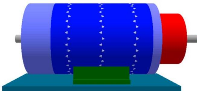
**Figure 6.** Water-cooled motor drawn using Motor-CAD.
