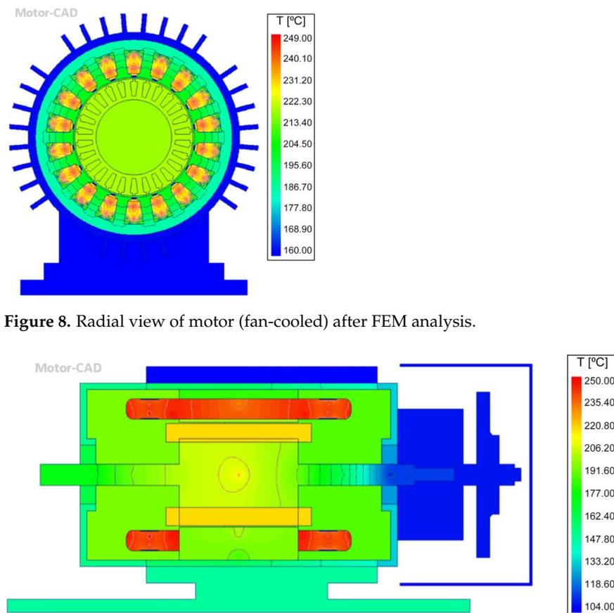
**Figure 8.** Radial view of motor (fan-cooled) after FEM analysis.
