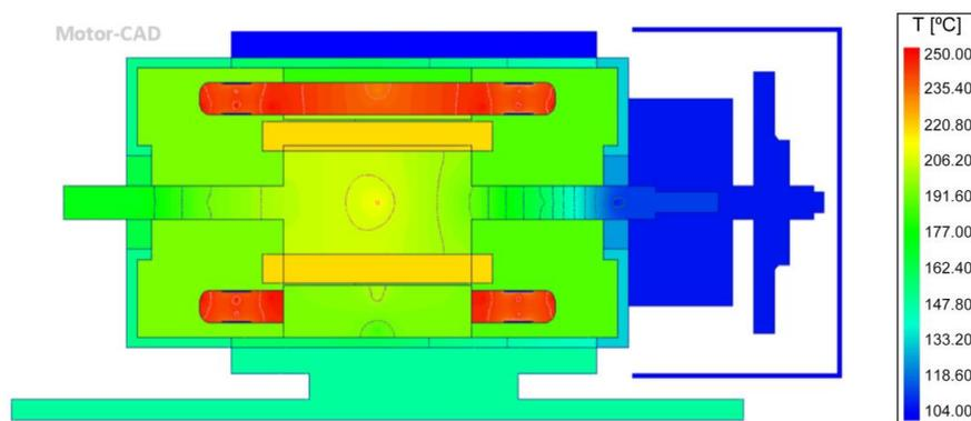
**Figure 9.** Axial view of motor (fan-cooled) after FEM analysis.
