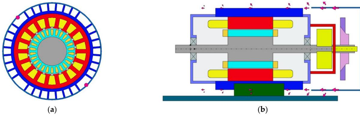
**Figure 7.** Radial view of fan-cooled motor mainly showcasing the housing type-axial fins (the windings, stator, and rotor) (a); axial view of fan-cooled motor depicting air flow coming from fan cooling system through the arrows (b).
