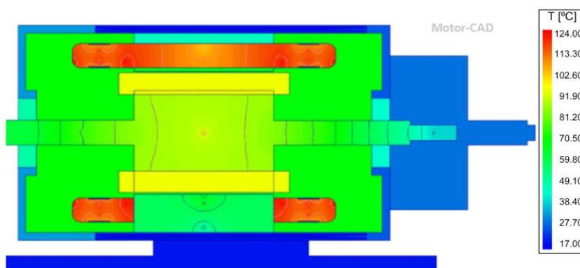
Figure 13. Axial view of water-cooled motor (aluminum casing) after the FEM analysis.
