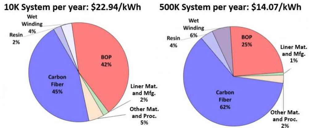
Figure 7. Cost breakdown of 70 MPa tank type IV system [145].
