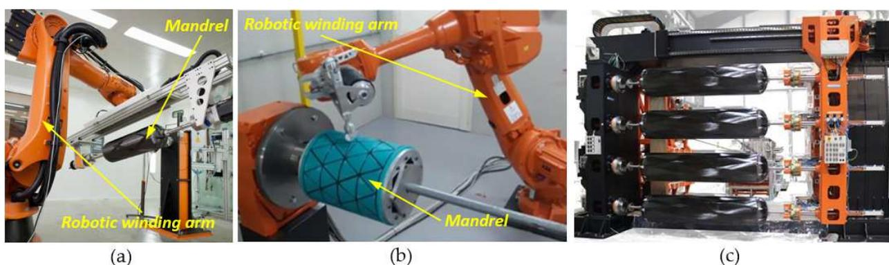
**Figure 5.** Arrangements of robot head installation: (a) fixed fiber guide/payout eye and flexible mandrel [119]; (b) flexible fiber guide/payout eye and fixed mandrel [118]; (c) Mikrosam's automated production line for CNG and hydrogen tanks [120]. Reproduced with permission from Mikrosam.
