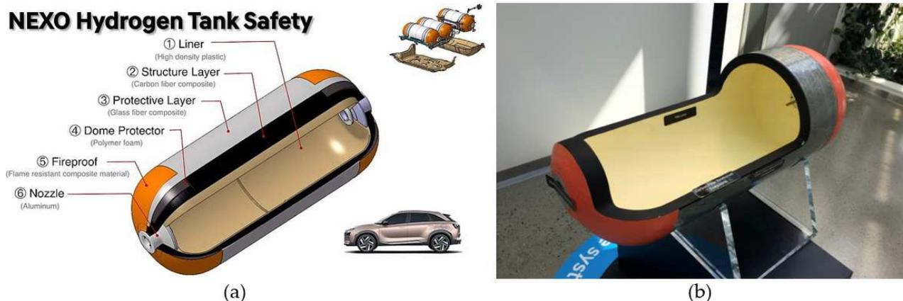
**Figure 1.** (a) Schematic cross-section of a hydrogen tank for Hyundai Nexo [18]; (b) photograph of a sectioned Hyundai Nexo hydrogen tank [19].
