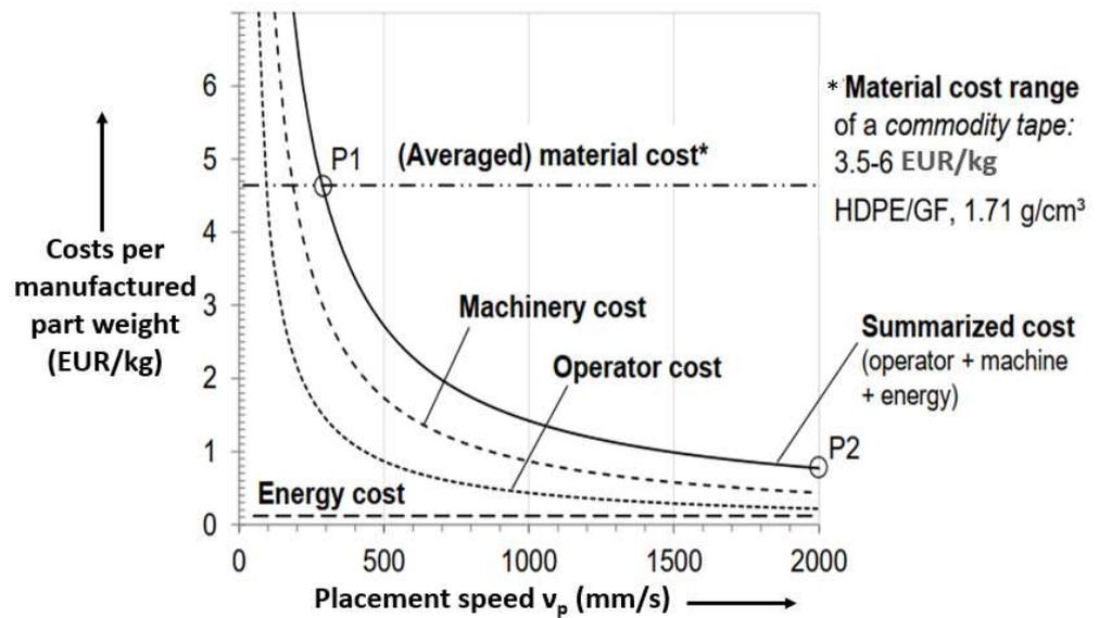
Figure 6. Breakdown of costs per produced part weight for various placement speeds [144].
