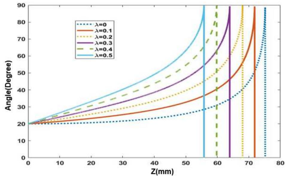
**Figure 10.** Influence of slippage coefficient on the turnaround radius of the non-geodesic path. By changing its value, turnaround radius of the helical path is changed.
