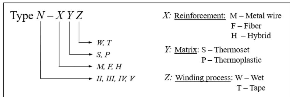
Figure 3. Classification for the sub-types of hydrogen tanks used in industrial applications.
