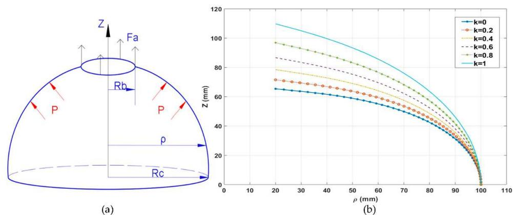
**Figure 9.** Dome design: (a) schematic representation of dome; (b) isotensoid dome contour generated with numerical integration.
