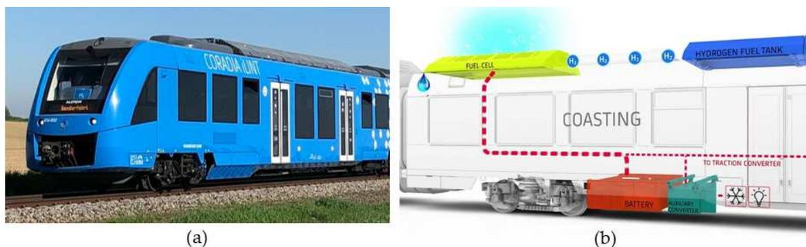
**Figure 2.** (a) Coradia iLint, the world's first hydrogen fuel cell passenger train [66]. Reproduced with permission from Alstom/R.Frampe; (b) Layout of FC train elements onboard [67].
