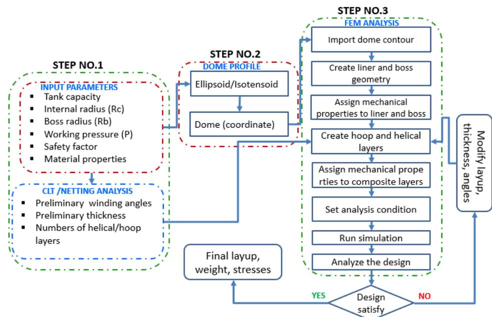
**Figure 8.** Flowchart of design and analysis of composite hydrogen tank.
