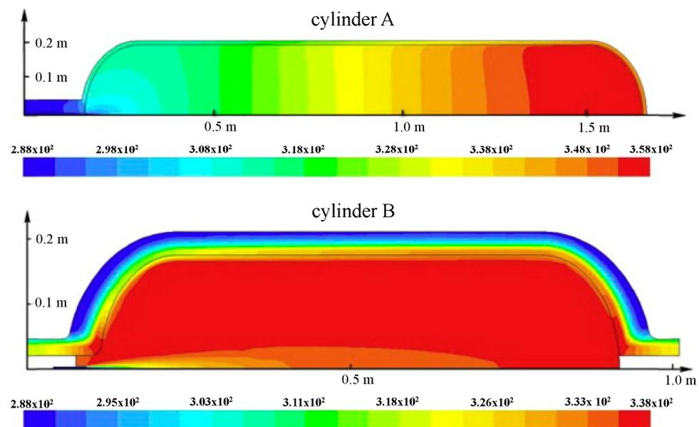
**Figure 11.** Hydrogen temperature distribution within the cylinder at the end of refueling [172]. Reprinted with permission from Zheng et al, International Journal of Hydrogen Energy, published by Elsevier, 2013.
