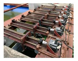
Figure 7. Wave-making system.
