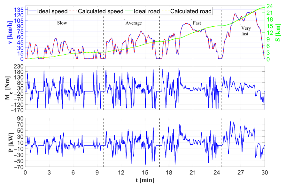
Figure 16. WLTP driving cycle for 2 \times 146 kW IPMSM in EV.
