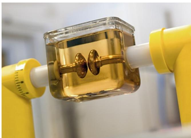
**Figure 13.** Dielectric breakdown voltage measurement test [57].
