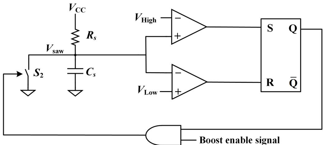
Figure 9. The sawtooth wave generation circuit.
