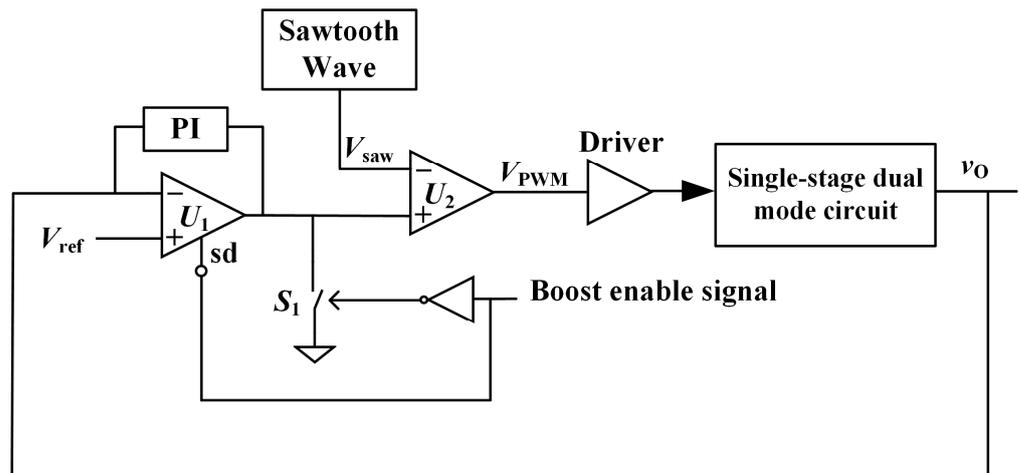
Figure 8. PI-regulated boost mode operation.
