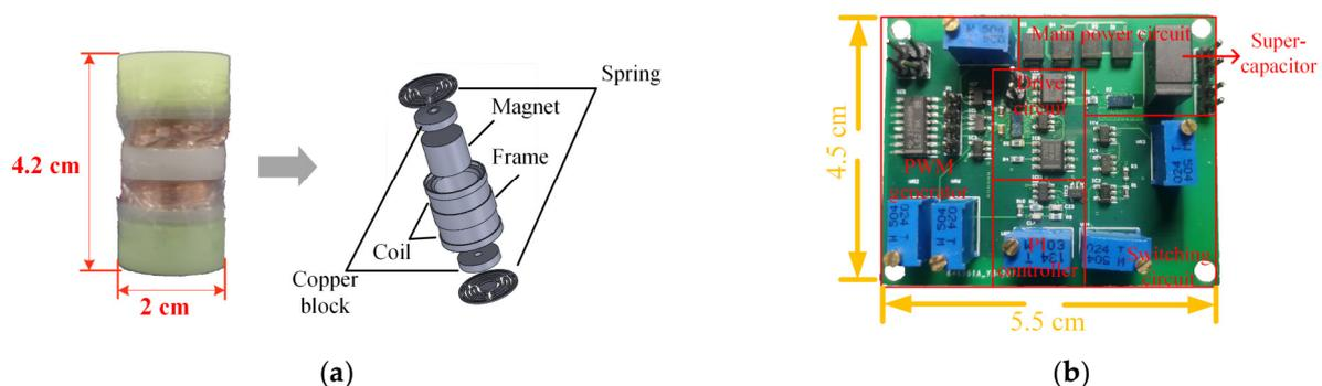
Figure 14. (a) The EVEH module used in the system [22]; (b) the prototype of the designed dual-mode hybrid step-up circuit.
