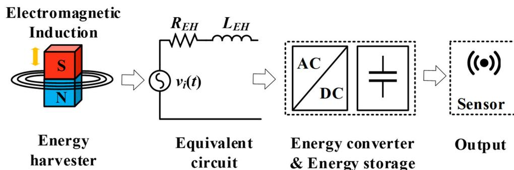
Figure 1. Basic architecture of electromagnetic EVEH.
