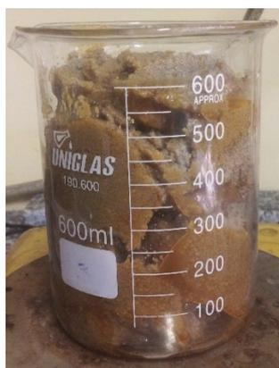
**Figure 2.** Pre-treated residual fat used as feed material by catalytic upgrading of residual fat vapors at 400 °C, 1.0 atm, 0.0%, 5.0%, 7.5%, and 10.0% (wt.) activated carbon pellets impregnated with 10.0 M NaOH, using a catalyst fixed-bed reactor, in semi-pilot scale.
