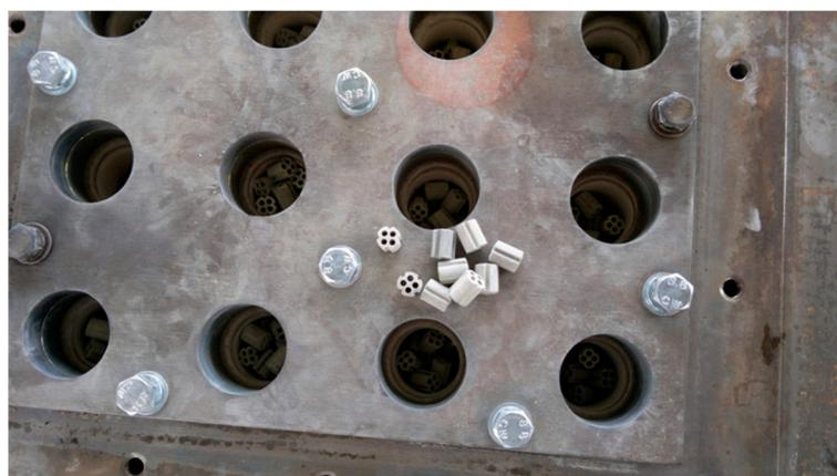
**Figure 4.** Detail of ceramic candles filled with quadralobe-shaped pellets of commercial Ni-catalyst for simultaneous product gas filtration and composition upgrading.
