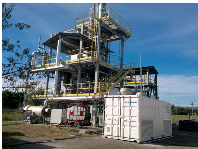
**Figure 3.** Gasifier coupled with the containerized PPS.
