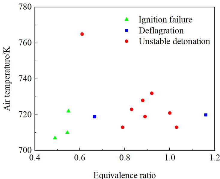
Figure 10. Modes’ distribution of liquid kerosene/hot air rotating detonation.
