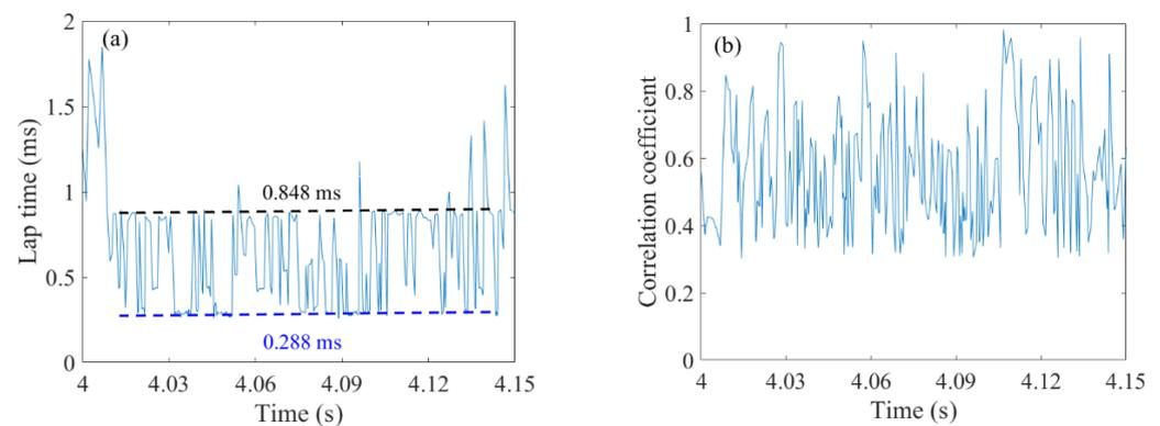
**Figure 6.** Autocorrelation results of B10 (4.0–4.16 s): (a) lap time and (b) correlation coefficient.
