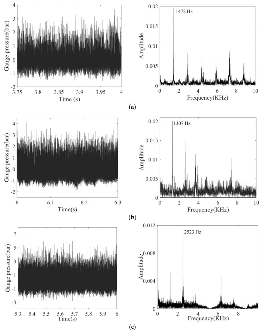
**Figure 2.** Local high–frequency pressure and FFT results of (a) Test A6, (b) Test A7, and (c) Test A5.
