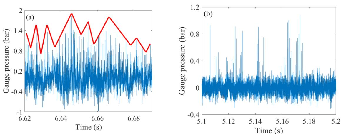
**Figure 9.** Instability phenomena: (a) low–frequency oscillation and (b) sporadic detonation.
