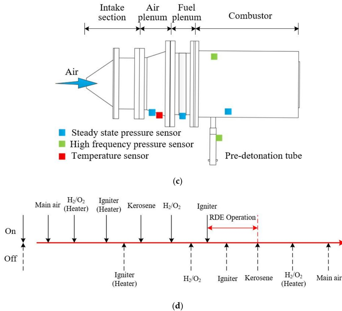
**Figure 1.** Overview map of experiments. (a) Schematic of the experimental system. (b) Injection scheme for kerosene. (c) Installation positions of sensors. (d) Time sequence of the experiments.
