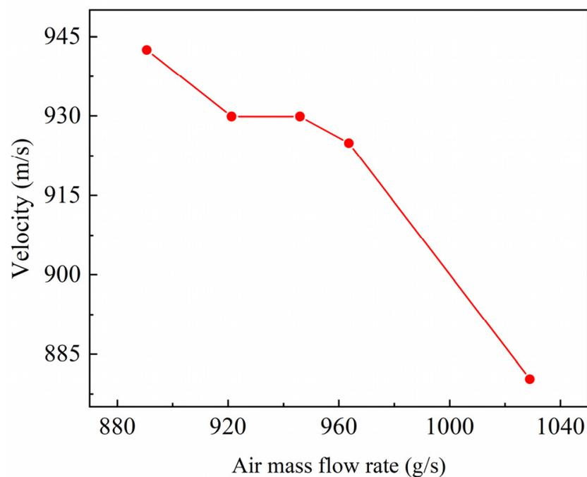
**Figure 3.** Variation of wave speed with air mass flow rate (mass fraction of H<sub>2</sub> 12%).
