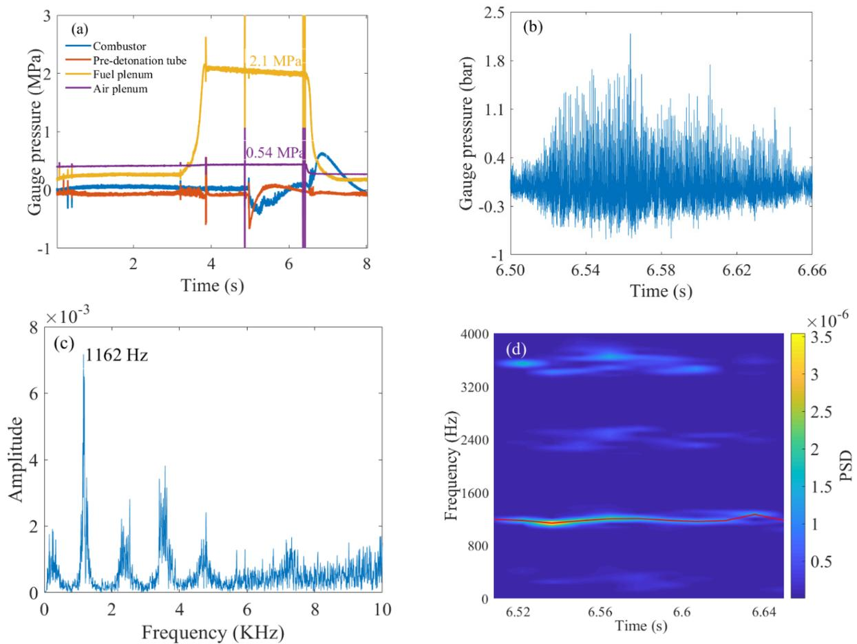
**Figure 4.** The rotating detonation experiment of B4: (a) original signal, (b) filtered signal, (c) frequency spectrum, and (d) time–frequency diagram.
