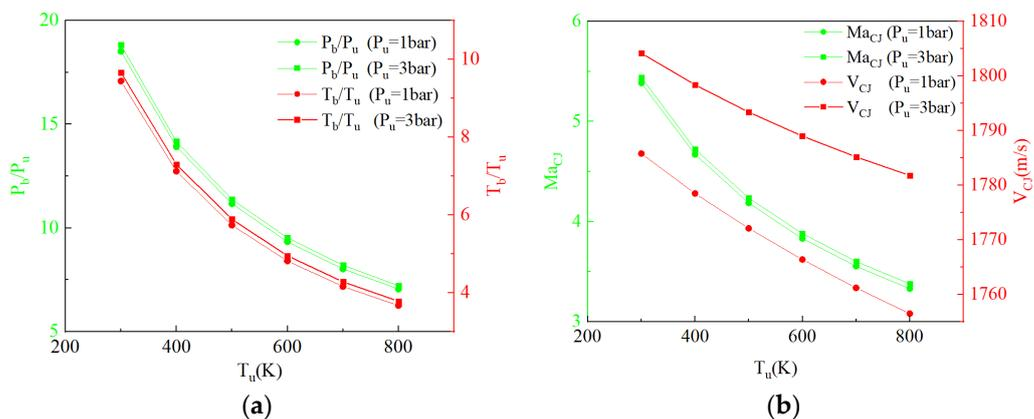
Figure 11. Effects of air temperature on intensity of detonation wave. (a) Static pressure ratios and static temperature ratios. (b) Mach number before detonation wave and wave velocity.
