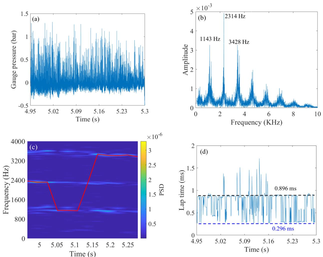
**Figure 8.** The rotating detonation experiment of B14: (a) filtered signal, (b) frequency spectrum, (c) time–frequency diagram, and (d) lap time.
