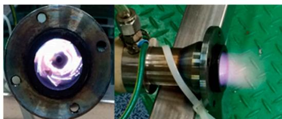
**Figure 2.** Direct photos of the plasma burner assisted SCR system.
