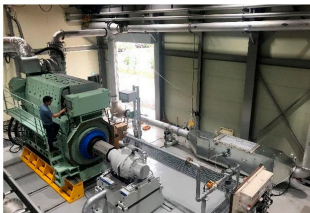
**Figure 4.** SCR system with a plasma burner.
