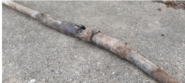
**Figure 1.** Example of damage to a cable joint mounted on a cable type XRUHAKXS 1 × 240/50.
