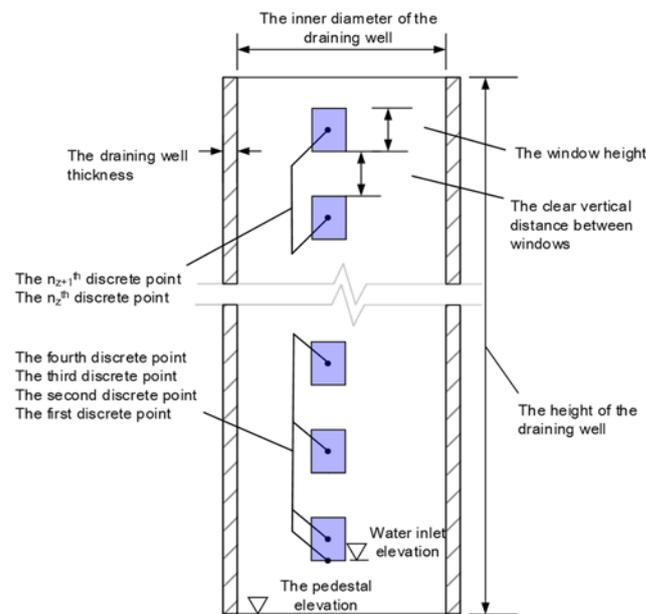
**Figure 3.** Water level discrete method.
