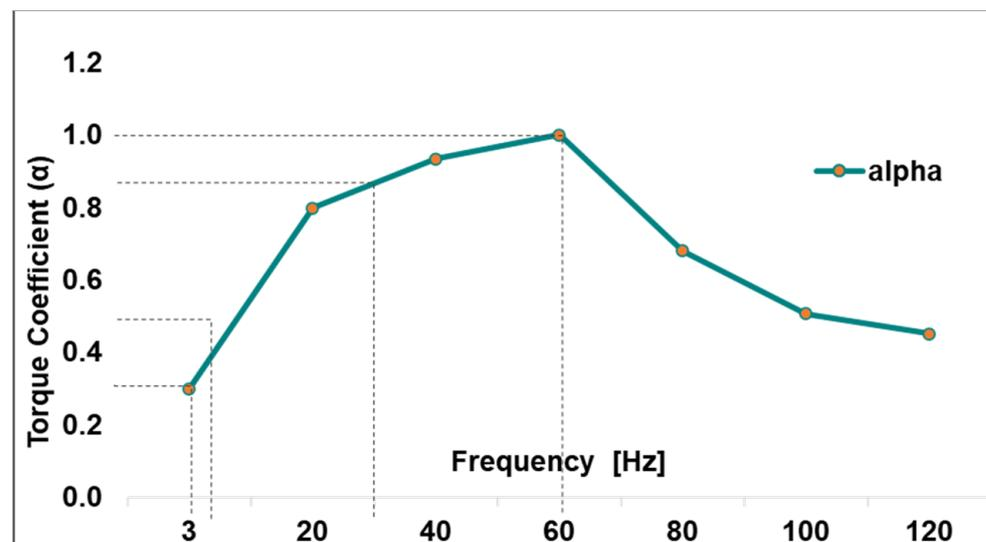
Figure 6. Torque coefficient curve of the V/F control induction motor used in this study.
