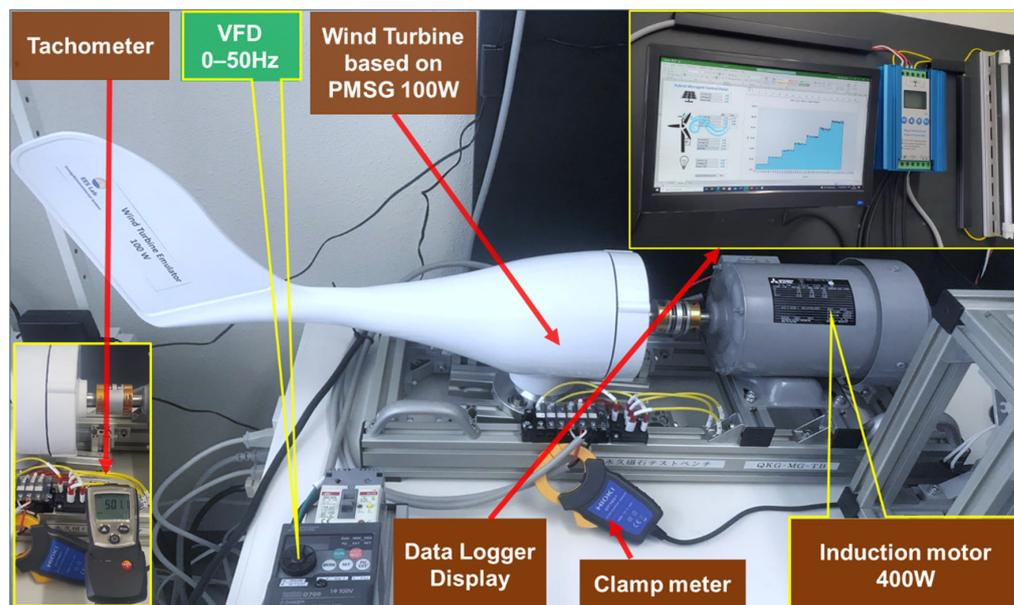
**Figure 5.** Wind turbine experimental setup in this study.
