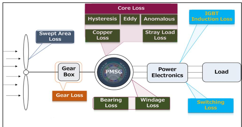
**Figure 1.** Wind turbine power train and types of distributed losses.
