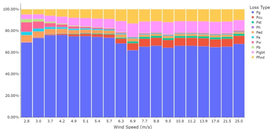
**Figure 9.** Distribution of the power loss in different stages of the indirect drive wind turbine.
