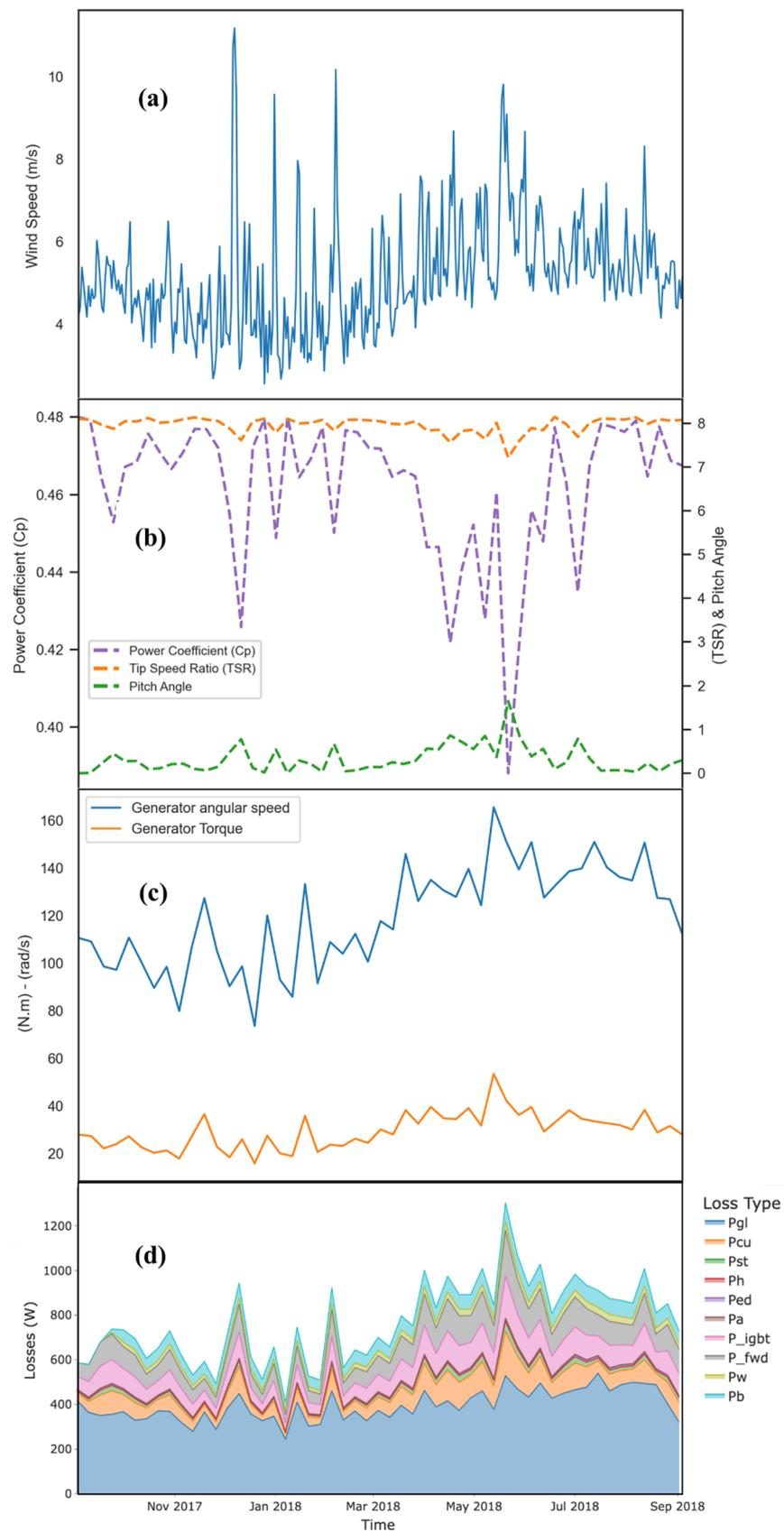
**Figure 10.** Model results for a 20 kW indirect drive wind turbine installed in Gwadar city: (a) wind speed, (b) behavior of decision variables, (c) generator torque and angular speed, and (d) power losses.
