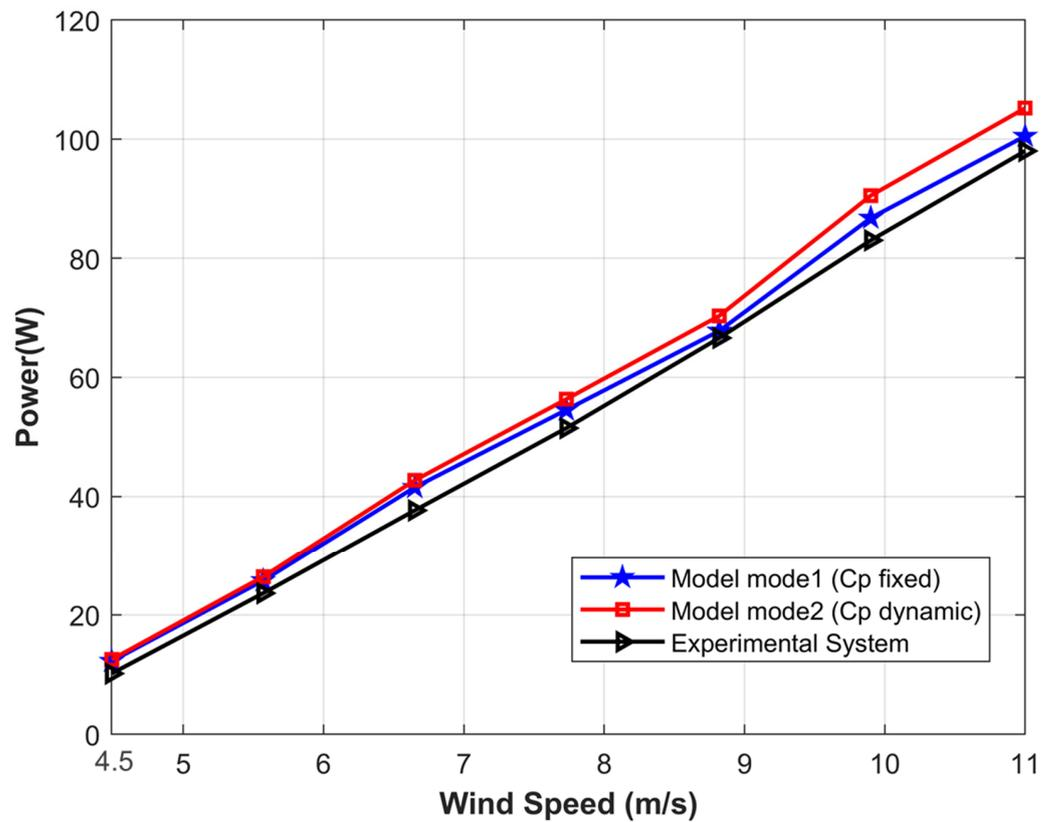
Figure 7. Comparison between the model results and measured data from the experimental setup in this study.
