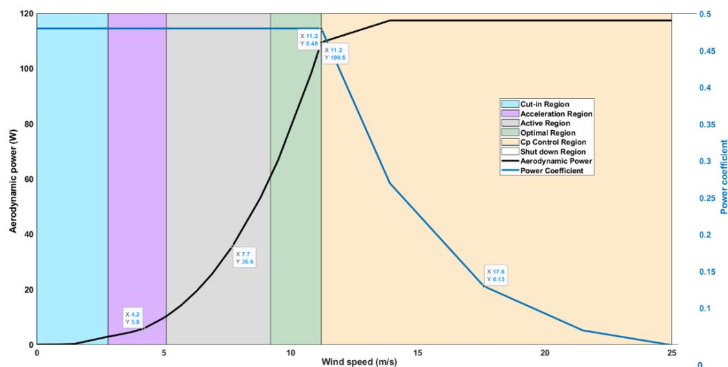
**Figure 2.** Variation of the optimal power coefficient with wind speed.
