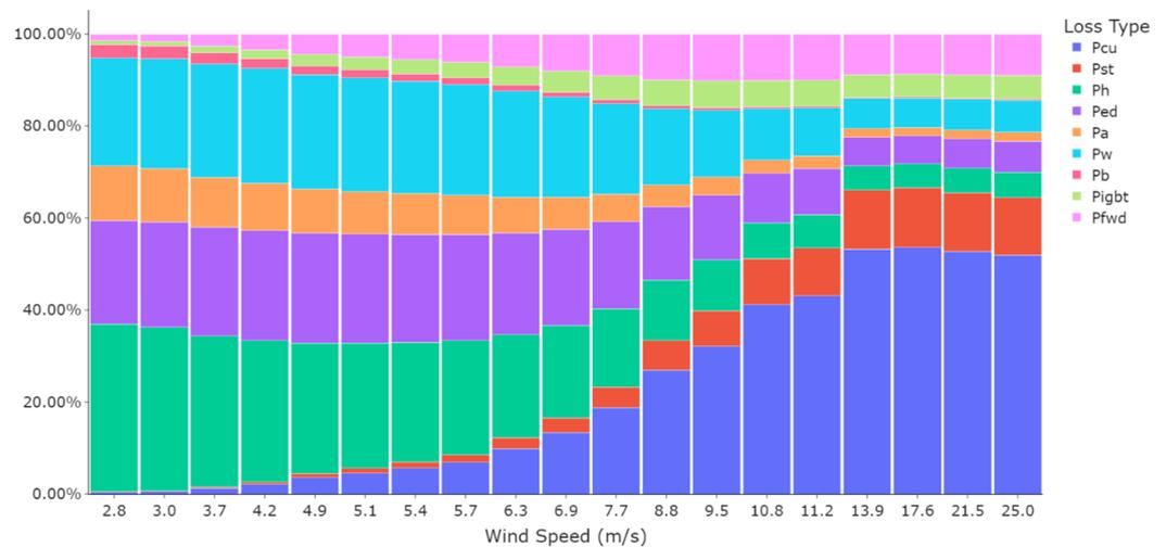
Figure 4. Distribution of the power losses in different stages of a direct-drive wind turbine.
