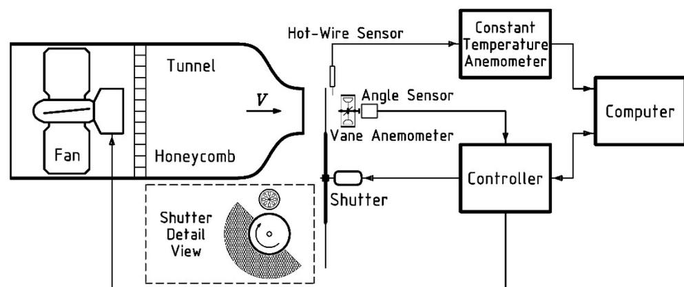
**Figure 1.** Diagram of the test stand.
