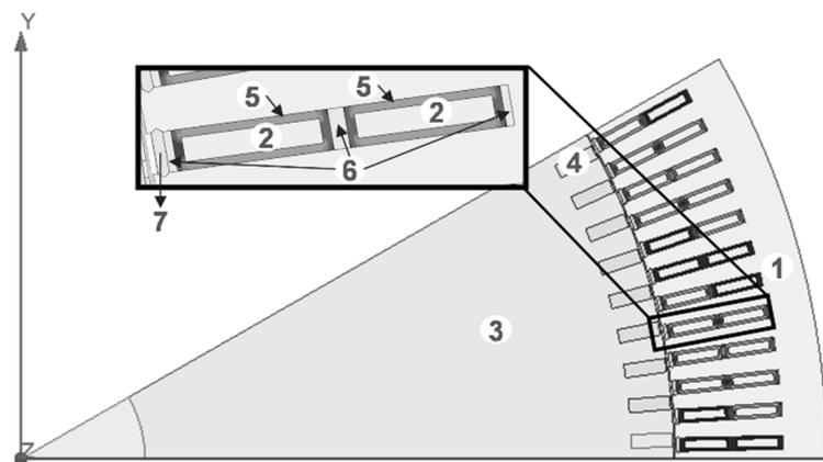
**Figure 9.** 2D FEA model of the medium-voltage machine. Different parts of the motor are numbered and listed in Table 3.
