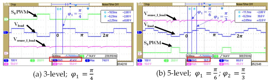
**Figure 18.** Experimental results—effect of increase in voltage levels.
