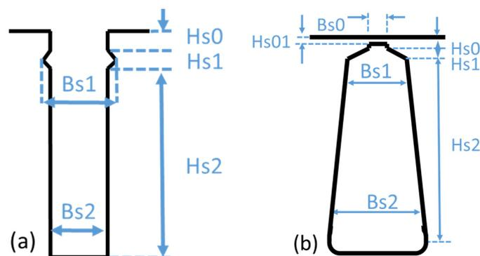
**Figure 7.** Parameters of a stator slot and a rotor slot. (a) Stator Slot dimensions. (b) Rotor Slot dimensions.
