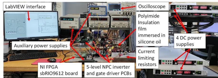
**Figure 15.** Experimental setup—NPC multilevel inverter.
