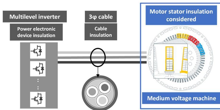
Figure 1. Medium-voltage machine drive with stator ground-wall insulation considered.
