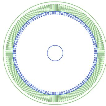
**Figure 8.** Ansys RMxprt model of medium voltage machine.
