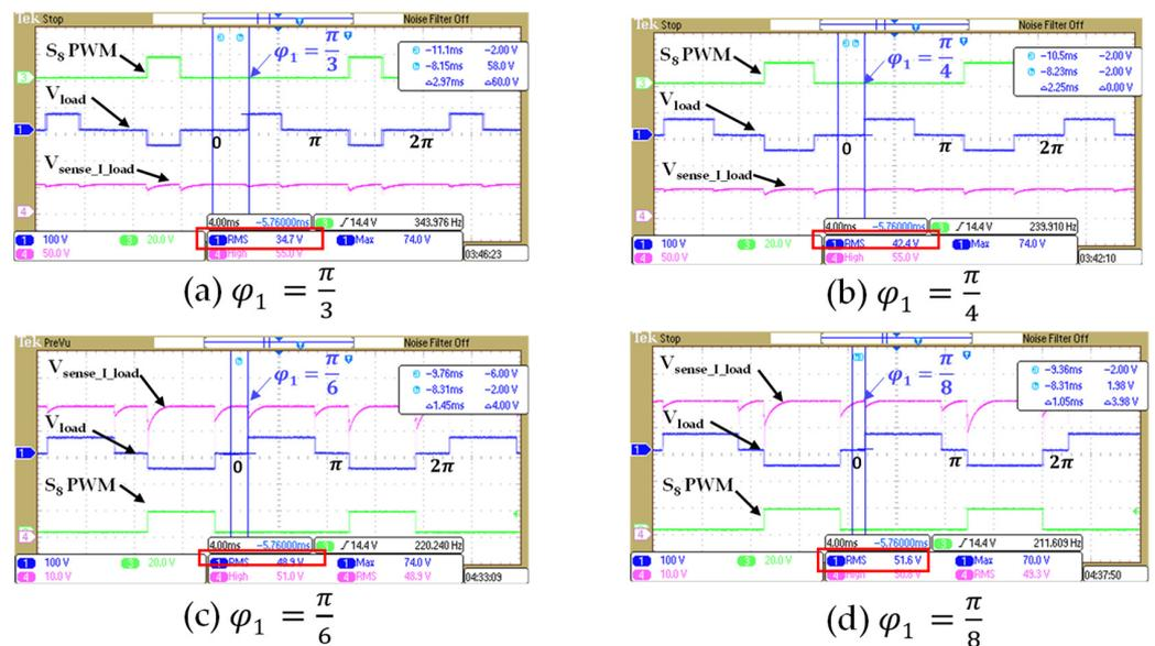
Figure 17. Experimental results—effect of increase in firing angles for 3-level inverter output.
