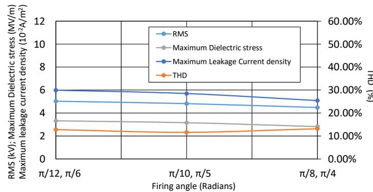
**Figure 12.** Effect of increasing firing angle in a 5-level inverter. Left Vertical axis: RMS in kV; Maximum Dielectric stress in MV/m; Maximum leakage current density in 10<sup>-2</sup> A/m<sup>2</sup>; Right Vertical axis: THD in %.
