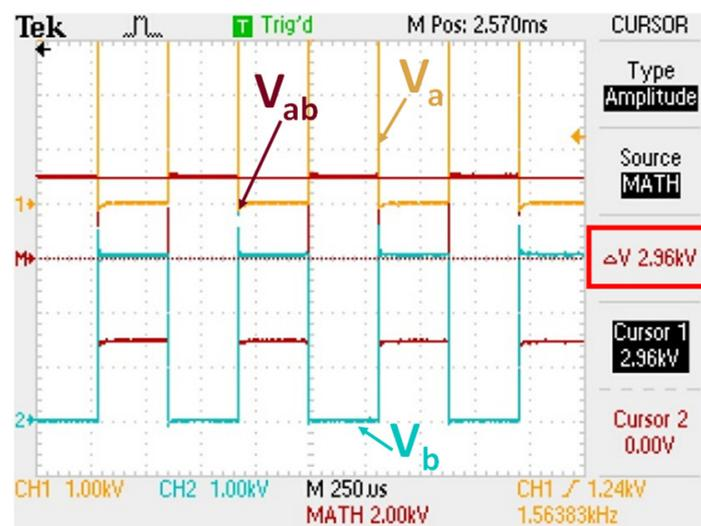
Figure 20. 2-level 3 kV peak medium-voltage inverter output.
