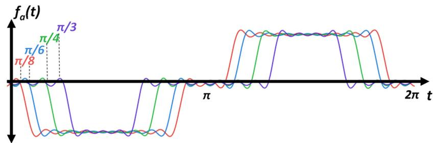
Figure 10. Effect of increasing firing angle in a 3-level inverter.
