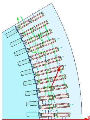
**Figure 3.** Zoomed-in contour of leakage current density vectors ( $\text{A}/\text{m}^2$ ).
