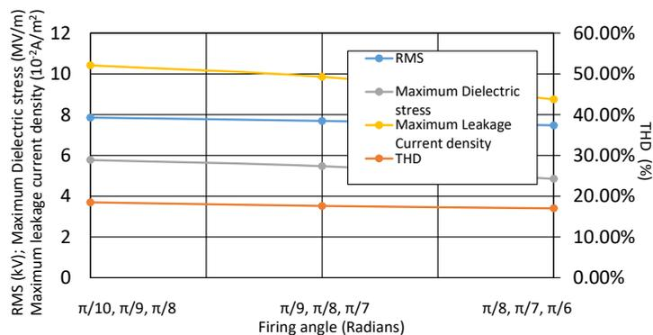
**Figure 13.** Effect of increasing firing angle in a 7-level inverter. Left Vertical axis: RMS in kV; Maximum Dielectric stress in MV/m; Maximum leakage current density in 10<sup>-2</sup> A/m<sup>2</sup>; Right Vertical axis: THD in %.
