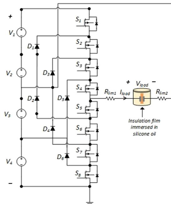
**Figure 14.** Schematic of a five-level NPC multilevel inverter used for experimental tests.
