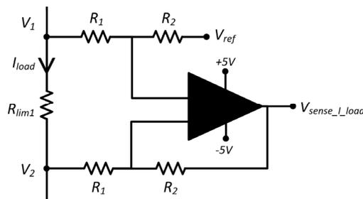
Figure 16. Differential amplifier circuit for leakage current measurement.
