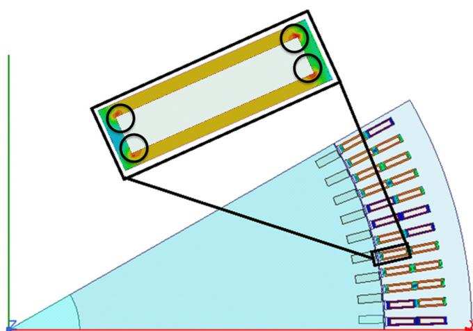
**Figure 2.** Contour of dielectric stress (V/m) in stator ground-wall insulation.
