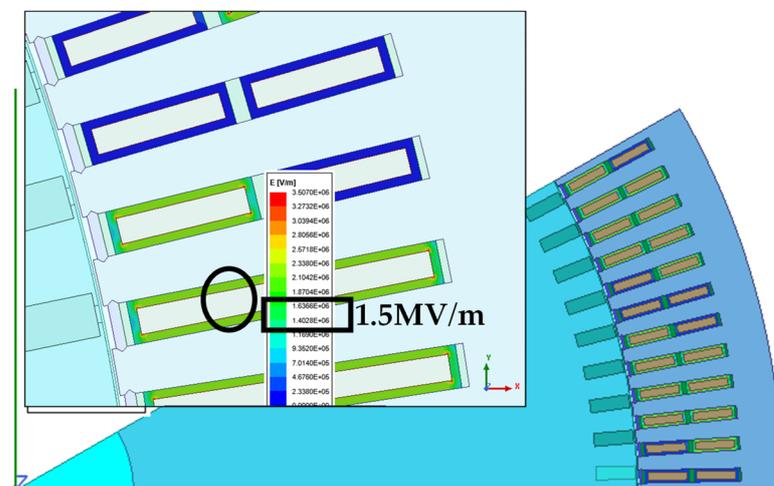
Figure 22. Dielectric stress within the motor stator winding matches the dielectric stress generated by 3 kV peak 2-level waveform using a hardware testbed.
