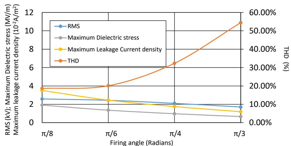
Figure 11. Effect of increasing firing angle in a 3-level inverter. Left Vertical axis: RMS in kV; Maximum Dielectric stress in MV/m; Maximum leakage current density in  $10^{-2} A/m^2$ ; Right Vertical axis: THD in %.
