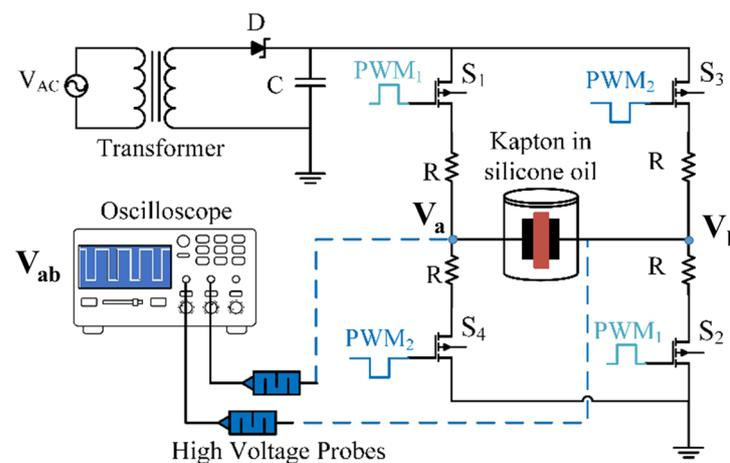
Figure 19. Schematic of 2 level medium-voltage inverter setup.
