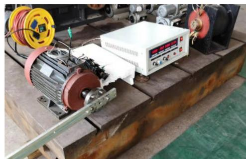
**Figure 26.** The inductance test of the prototype.
