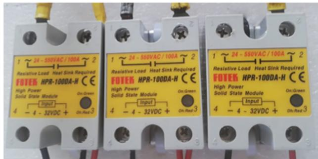
Figure 27. Solid state breakers used.
