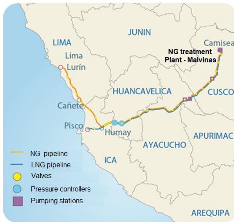
Figure 3. NG Transportation network (extracted from Osinergmin).
