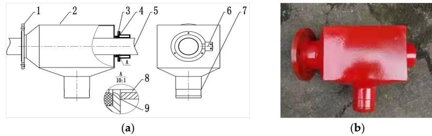
**Figure 2.** Structure of the dust hood: (a) structure chart: 1—mounting flange of the dust hood; 2—cavity of the dust hood; 3—unidirectional sealing ring; 4—dust control device; 5—drill pipe; 6—compressed air interface; 7—dust hood outlet; 8—gap between the drill pipe and the dust hood; 9—air slot of the sealing device; (b) real product.
