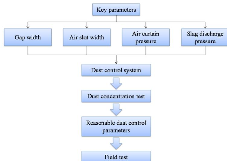
**Figure 4.** Parameter optimization process of dust control system.
