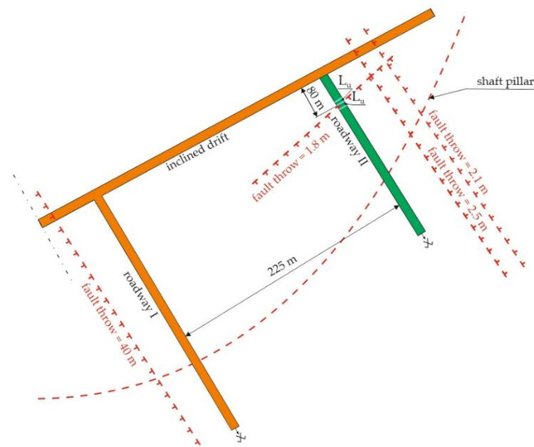
**Figure 4.** The area of the roadway with marked faults.
