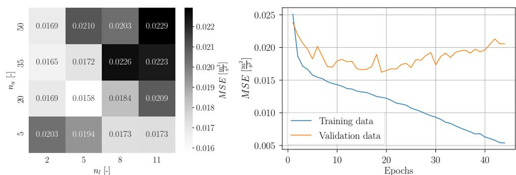
Figure 41. Visualization of the grid search results for adjusted  $n_{in}$  and  $n_{out}$  (left) and the learning curve of a subsequent training for  $n_l = 5$  and  $n_u = 20$  (right).
