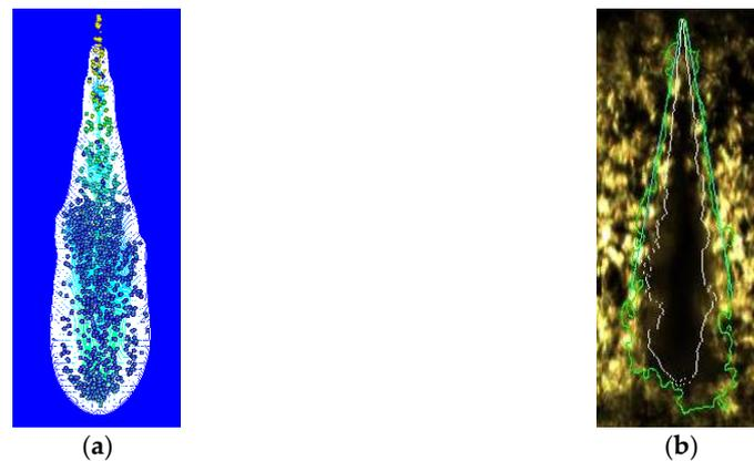
**Figure 7.** Comparison of the spray shape at 0.9 ms for Case 1. (a) Liquid- and vapor-phase spray of simulation; (b) Liquid- and vapor-phase spray of experiments.
