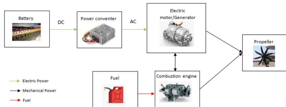
**Figure 3.** Series-parallel architecture. Source: Processed by authors.
