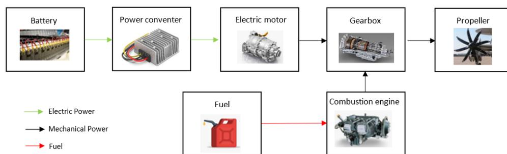
**Figure 1.** Parallel hybrid architecture. Source: Processed by authors.
