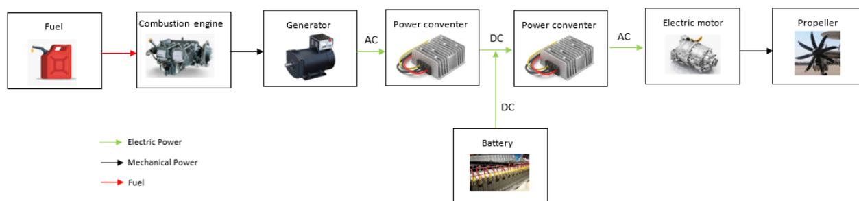
**Figure 2.** Serial hybrid architecture. Source: Processed by authors.
