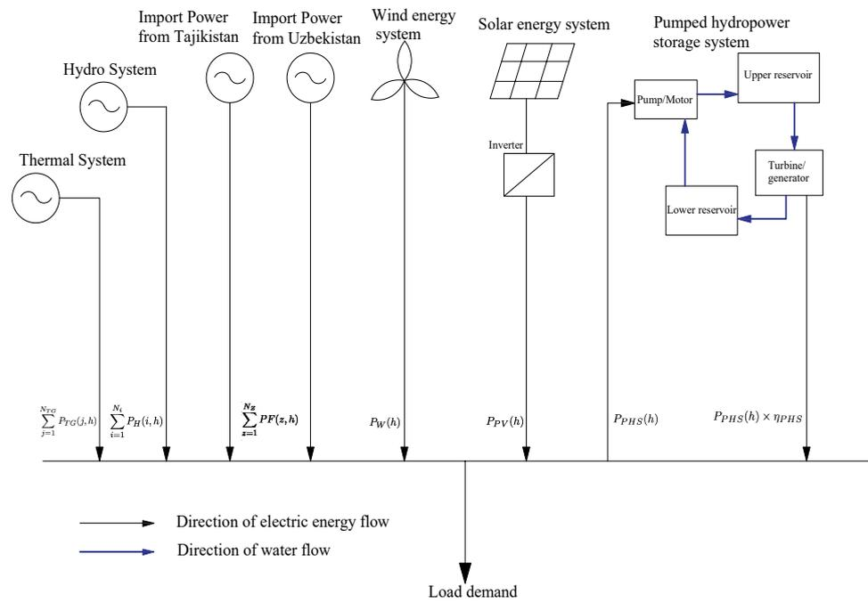
Figure 6. The generation system under study.
