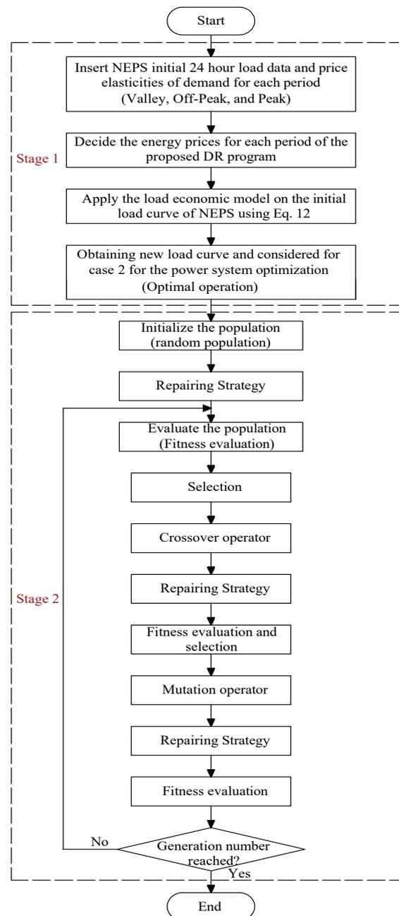
Figure 5. Flowchart of the proposed methodology used in this study.
