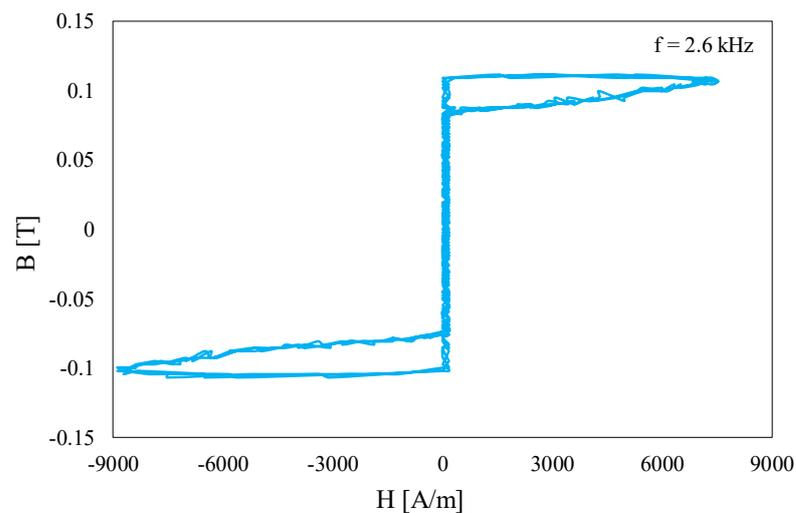
**Figure 8.** Hysteresis loop of the investigated nanocrystalline core.
