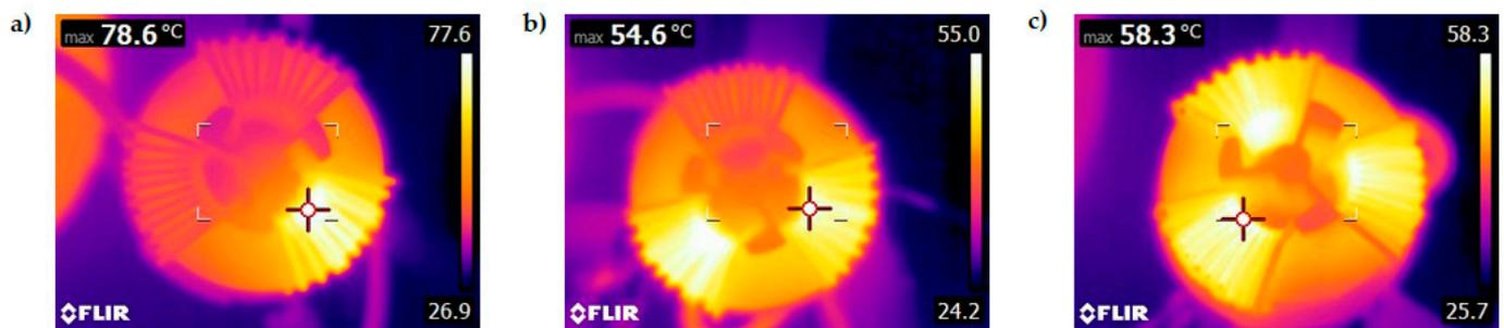
Figure 10. Thermograms illustrating the temperature distribution in the inductor when the current flows through one winding (a), two windings connected in series (b), and three windings connected in series (c).
