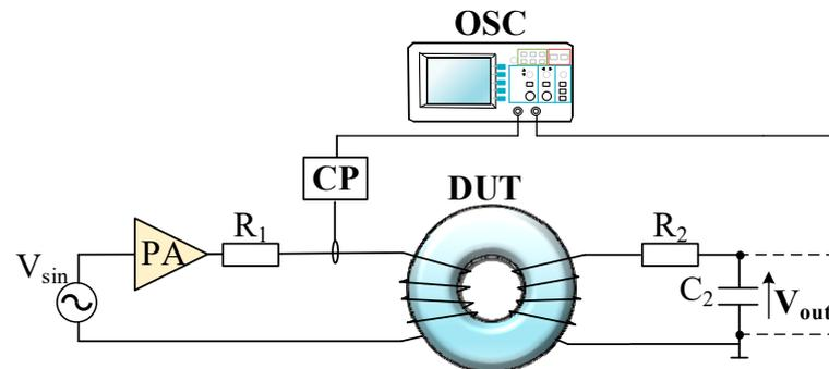
**Figure 7.** Setup to measure the hysteresis loop.
