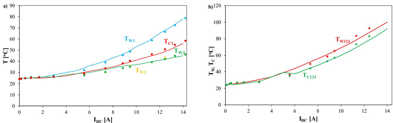
**Figure 14.** Dependence of the temperature of the inductor components on the direct current (a) when power is dissipated in one winding, (b) when the power is dissipated in three series-connected windings.
