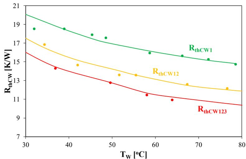
**Figure 12.** Dependence of mutual thermal resistance between the inductor core and the winding on the winding temperature for one, two, and three series-connected windings.
