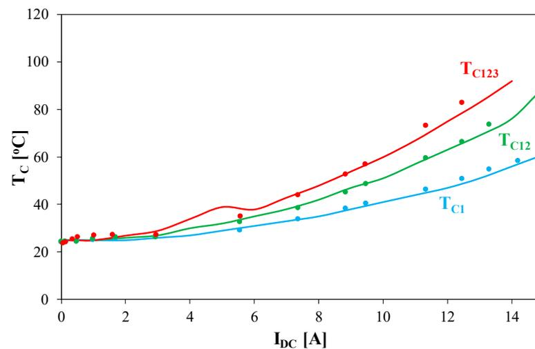
**Figure 15.** Dependence of the inductor core temperature on the direct current  $I_{DC}$  when the current flows through one, two, or three windings connected in series.
