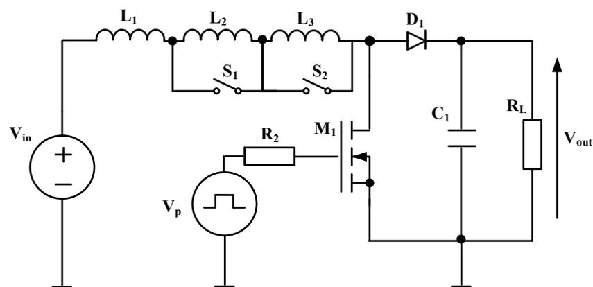
**Figure 17.** Analysed circuit of a boost converter.
