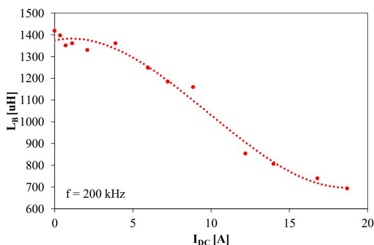
**Figure 6.** Dependence of the blocking inductance  $L_B$  of a blocking inductor on the direct current  $I_{DC}$ .
