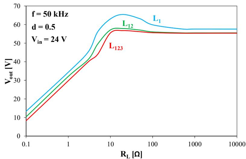
**Figure 18.** Dependence of the output voltage on the load resistance of the boost converter when the current flows through one coil, two coils, or three coils connected in series.
