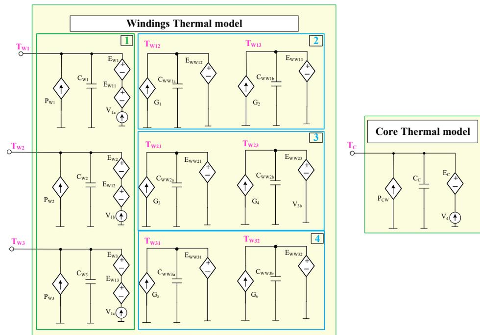
Figure 2. Network representation of the thermal model of a coupled inductor.
