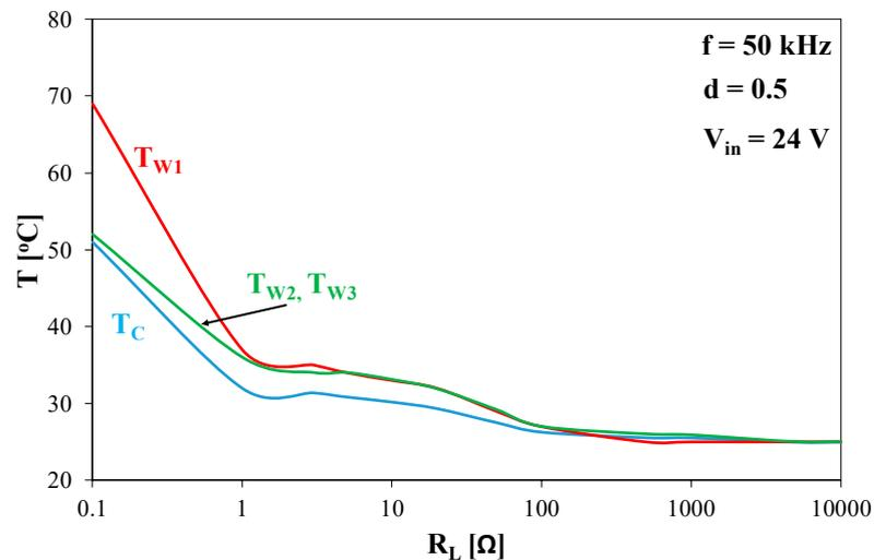
**Figure 19.** Dependence of the core and winding temperature on the load resistance of the boost converter when the current flows through one coil.
