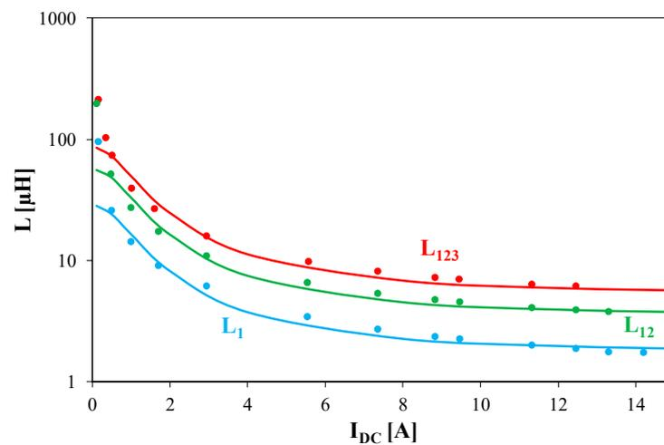
Figure 9. Dependence of inductance  $L_1$ ,  $L_{12}$ , and  $L_{123}$  on the direct current  $I_{DC}$  at  $f = 200$  kHz.
