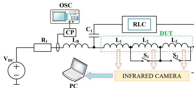
Figure 4. Setup for measuring the inductance of a coupled inductor using the LCR bridge.
