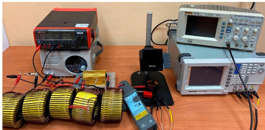
Figure 5. Photo of the setup for measuring the inductance of the inductor.
