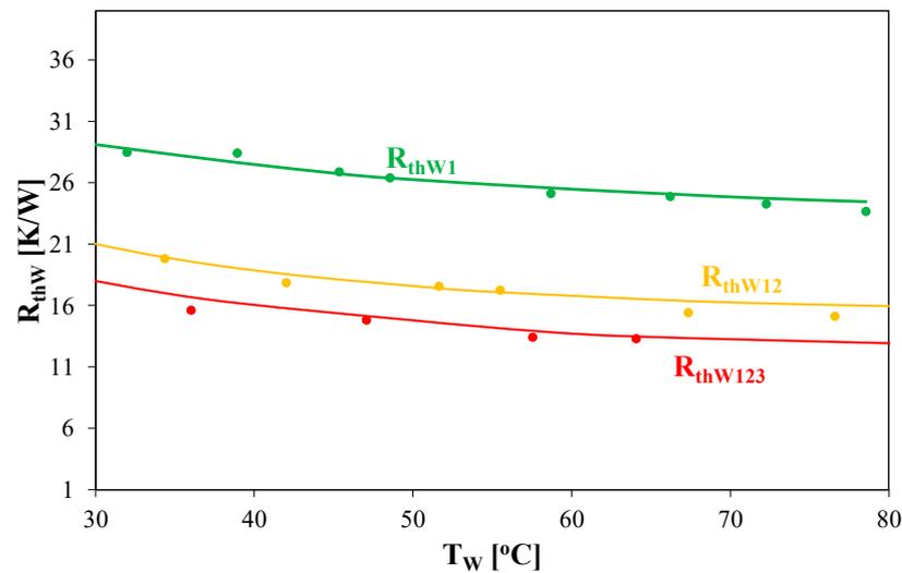
**Figure 13.** Dependence of thermal resistance of the inductor windings on the temperature of these windings  $T_{W1}$  with various number of powered windings at the same time.
