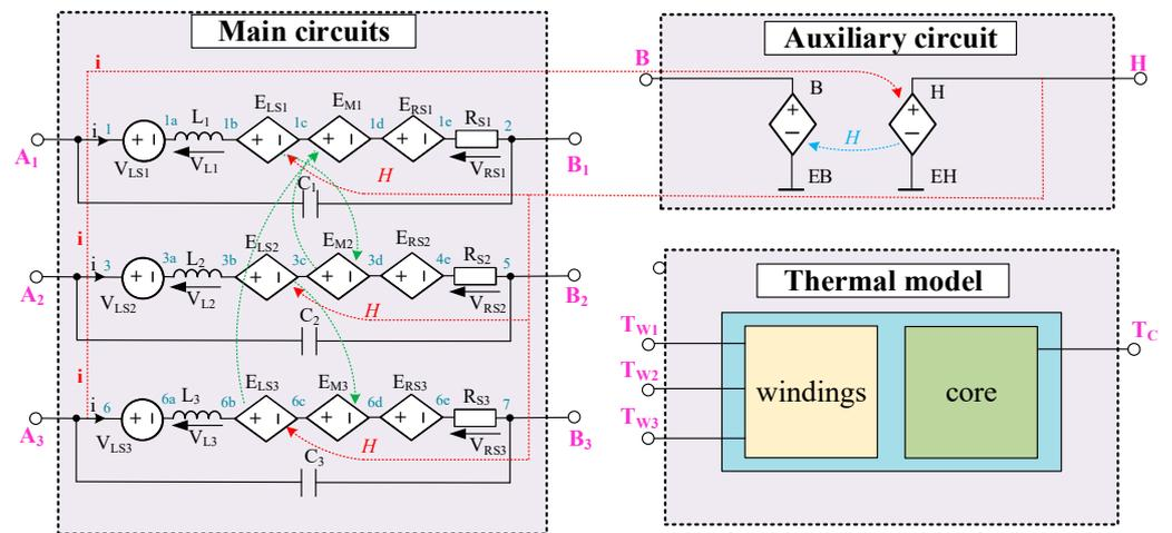
Figure 1. Network representation of an electrothermal model of a coupled inductor.
