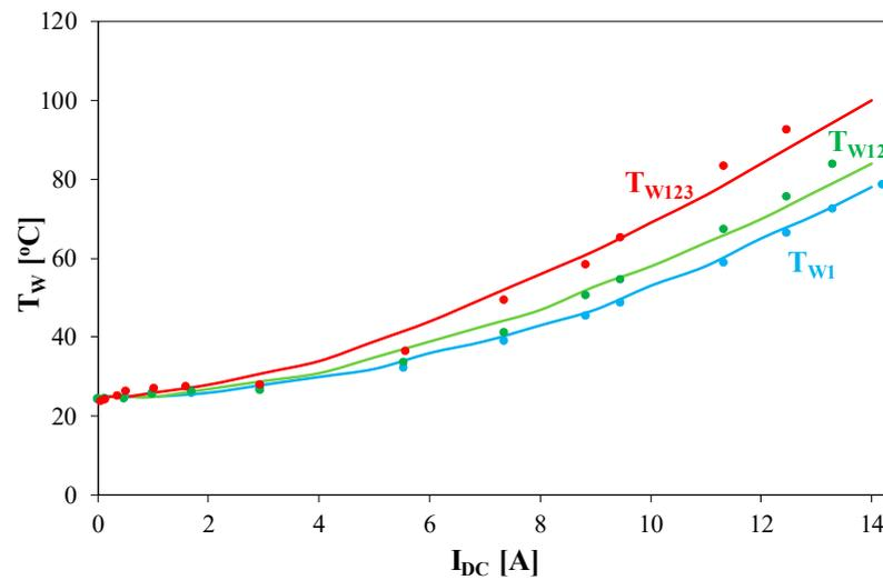
**Figure 16.** Dependence of the inductor winding temperature on the direct current  $I_{DC}$  flowing through one  $T_{W1}$ , two  $T_{W12}$ , or three  $T_{W123}$  windings connected in series.
