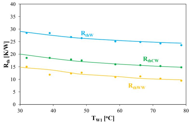
**Figure 11.** Dependence of thermal resistances of the inductor components on the temperature of the winding in which the power is dissipated.
