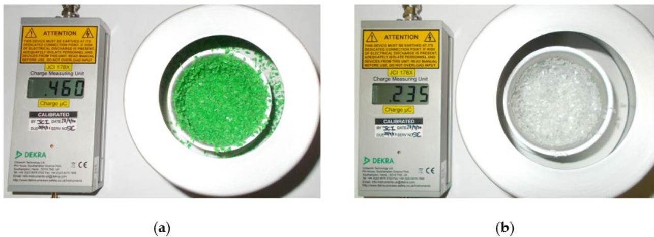
Figure 4. A system for measuring the accumulated charge on particles of (a) PE-HD and (b) PET polymers.
