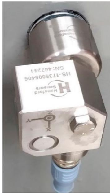
**Figure 2.** The Hansford Sensors piezoelectric accelerometer (model 1735005406) which was used during the measurements.
