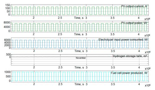
**Figure 20.** The result of the simulation and calculation of the required hydrogen tank capacity for the location Manipal, India (April only).
