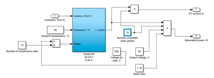
**Figure 15.** The array of 10 solar modules gives the output power.
