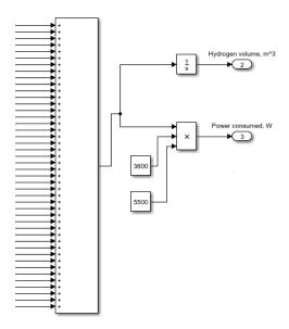
Figure 9. The subsystem of the electrolyzer cell stack (place 'A').
