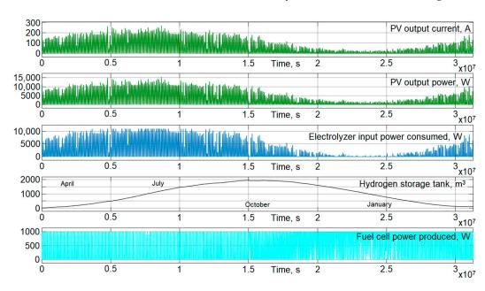
**Figure 17.** The result of the simulation and calculation of the required hydrogen tank capacity for the location Chelyabinsk, Russia.
