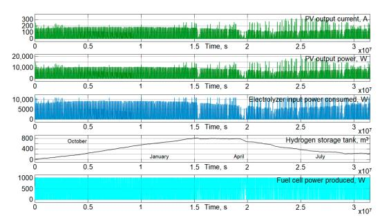
**Figure 21.** The result of the simulation and calculation of the required hydrogen tank capacity for the location Gnaraloo, Australia.
