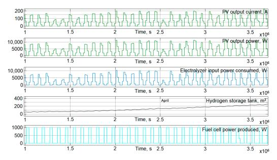
**Figure 18.** The result of the simulation and calculation of the required hydrogen tank capacity for the location Chelyabinsk, Russia (April only).
