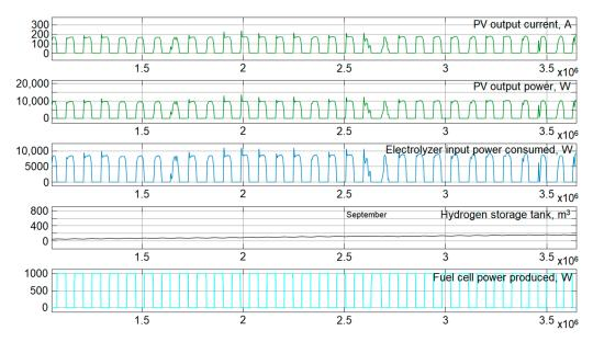
**Figure 22.** The result of the simulation and calculation of the required hydrogen tank capacity for the location Gnaraloo, Australia (April only).
