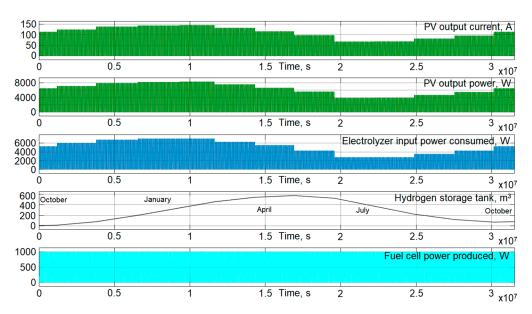
**Figure 19.** The result of the simulation and calculation of the required hydrogen tank capacity for the location Manipal, India.
