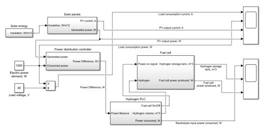
**Figure 13.** The complete model of the photovoltaic powered hydrogen generation system in Matlab/Simulink.
