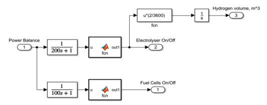
Figure 7. The subsystem of the electrolyzer.
