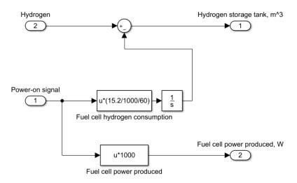
Figure 12. Hydrogen production and pumping for fuel cell operation.
